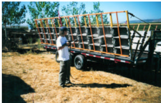
Figure 12: Portable trailer-based container wash rack.
