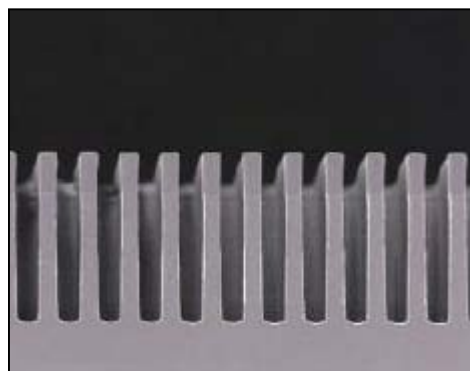
Etched Trenches 10 \mu\text{m} features, 65 \mu\text{m} deep (Photo Courtesy of ULVAC)
