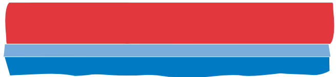
Coat and Softbake Imaging Resist
