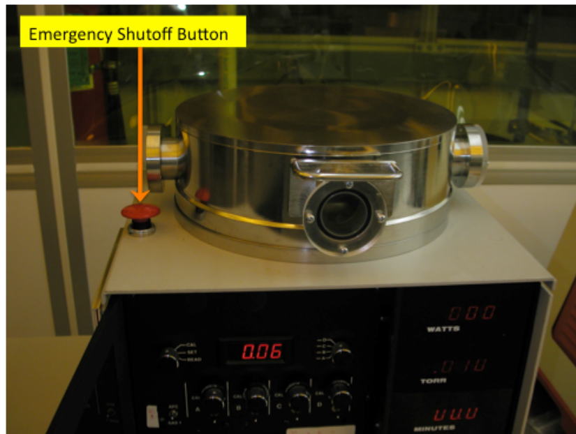
Figure 2: Emergency Shutoff Button
