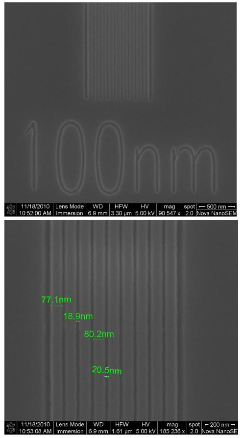
Pattern Name: Lines&Spaces Film Thickness: 125nm Pitch: 77.4nm Resolution: 15.9nm Energy (Area Dose): 245µC/cm<sup>2</sup> Energy (Line Dose): 0.12162nC/cm
