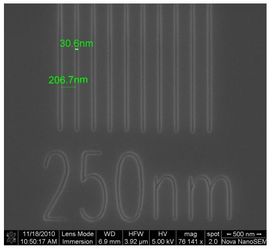
Pattern Name: Line&Spaces Film Thickness: 125nm Pitch: 151.7nm Resolution: 26.2nm Energy (Area Dose): 245µC/cm<sup>2</sup> Energy (Line Dose): 0.12162nC/cm
