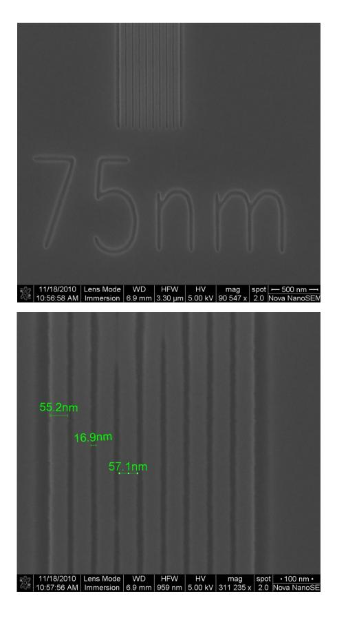
Pattern Name: Lines & SpacesFilm Thickness: 125nmPitch: 74.1nmResolution: 17.7nmEnergy (Area Dose): 245µC/cm²Energy (Line Dose): 0.12162nC/cm
