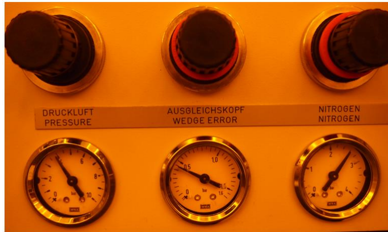
Figure 20 Image of pressure meters and regulators.
