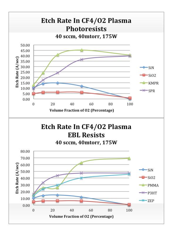
CF4/O2 plasmas find common use in etching Silicon Oxide and Silicon Nitride using a polymeric resist for patterning. Typical recipes utilize 5-15% O2 in the plasma. Though the chart shows data for a pure O2 plasma, please do not ash bulk resists in the PlasmaTherm.
