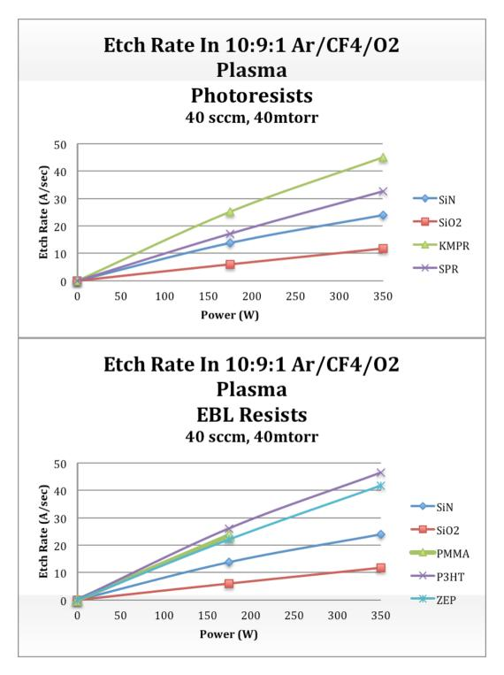
The PlasmaTherm controls platen bias with RF power. Etch rates show a linear dependence on RF power at 40mtorr.
