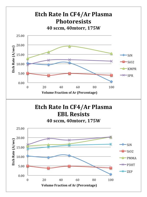
Diluting the plasma with Argon reportedly reduces the amount of grass formed while not reducing resist selectivity as much as Oxygen does. Including as much as 50% Argon did not drastically change etch rates for most materials.
