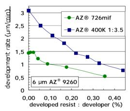
developed resist is solved in the developer, the development rate already drops by some 10 %, and the developer should be renewed. When the ratio resist : developer increases towards 1 %, almost all OH<sup>-</sup>-ions are consumed, and the development drops towards zero.
