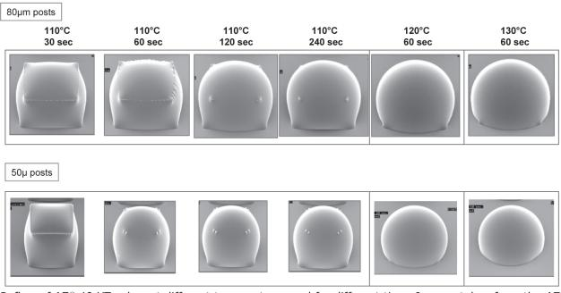
Reflow of AZ<sup>®</sup> 40 XT cubes at different temperatures and for different time. Images taken from the AZ 40XT-11D Thermal Flow data sheet of AZ-EM.
