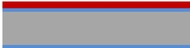
Figure 2 Substrate coated with 1.3 \mu\text{m} of S1813 positive photoresist.
