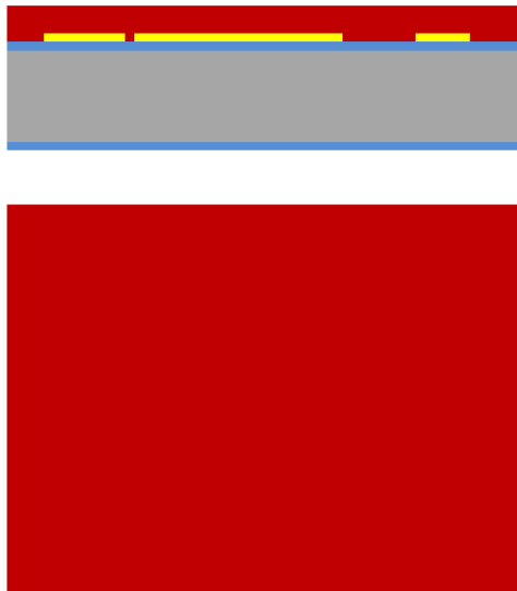
Figure 6 Substrate coated in photoresist.
