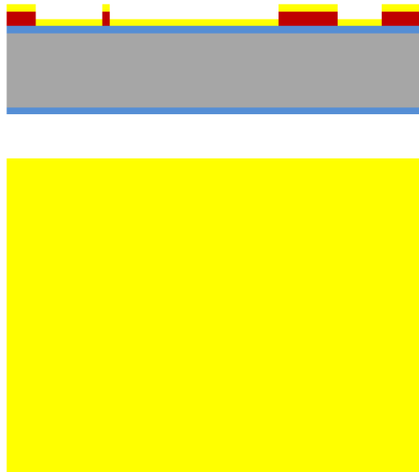
Figure 4 Substrate coated with 50 nm of chromium and 200-300 nm of gold using Lesker Sputter deposition.
