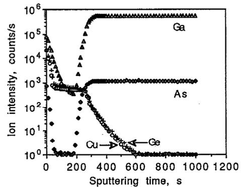
FIG. 5. SIMS profiles of an  $\epsilon_1$ -Cu<sub>3</sub>Ge/GaAs contact formed at 400 °C for 30 min. Note that only Ga has diffused into the  $\epsilon_1$ -phase alloy. The As signal in the  $\epsilon_1$ -phase alloy is at the background level.
