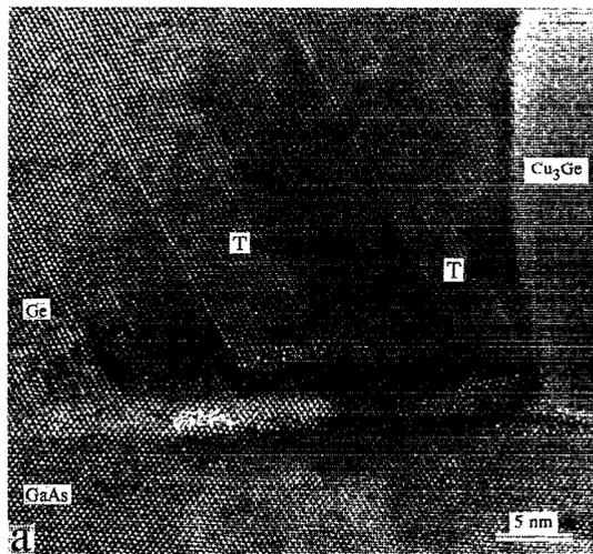
FIG. 2. (a) High-resolution TEM image showing the interface between a large epitaxial Ge grain and the GaAs substrate. Typical twin lamella are denoted by T. Arrow indicates an amorphous pocket at the interface. (b) Corresponding SAD pattern showing the [110] zone axis pattern of GaAs and Ge (unresolved) with typical twin spots (denoted by T).
