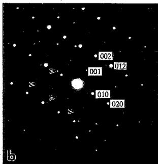
FIG. 4. (a) High-resolution TEM image of  $\epsilon_1$ -Cu<sub>3</sub>Ge/GaAs interface. The specimen is tilted into the [100] zone axis of the Cu<sub>3</sub>Ge phase, and GaAs is 5°–8° out of the [110] zone axis. (b) Corresponding SAD pattern. Spots of [100]-oriented  $\epsilon_1$ -Cu<sub>3</sub>Ge are indexed. Arrows aim at the GaAs spots. Reflexes denoted by asterisks correspond to a neighboring  $\epsilon_1$ -Cu<sub>3</sub>Ge grain.
