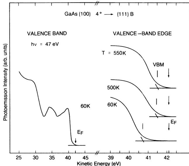
FIG. 2. SXPS valence-band spectra of a clean, misoriented GaAs (100)  $4^\circ \rightarrow [111]B$  surface at the indicated temperatures, exhibiting characteristic clean-surface features. The extrapolated valence-band edge moves closer to the Fermi level (arrow) with increasing temperature.
