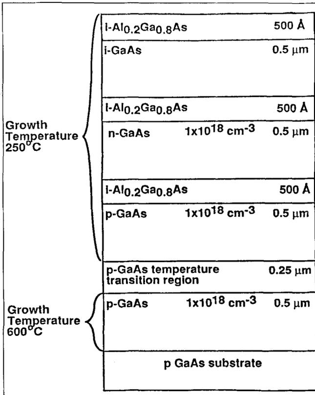
Fig. 1. Configuration of the p-n-i layer structure.
