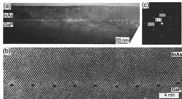
FIG. 4.  $\langle 011 \rangle$  XTEM micrographs of a 25-nm-thick InAs epilayer grown on GaP under In-stable conditions: (a) a HRTEM image showing that the epilayer has a relatively smooth surface with very few defects detected, (b) a HRTEM image revealing an incoherent interface with a series of 4 nm-spaced 90° misfit dislocations (arrowed), (c) an electron diffraction pattern taken from the interface area indicating a strain relaxed InAs epilayer in perfect epitaxial relationship with GaP.
