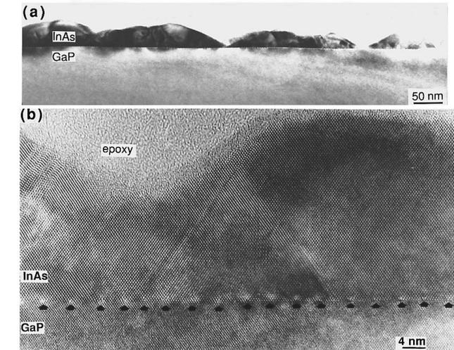
FIG. 3.  $\langle 011 \rangle$  cross-sectional (a) bright field and (b) HRTEM images of a 25-nm-thick InAs epilayer grown on GaP under As-stable conditions showing 3D islanding and a regular array of 90° misfit dislocations (arrowed) right at the heterointerface. Stacking faults are observed at the joint of two islands, indicating island coalescence.
