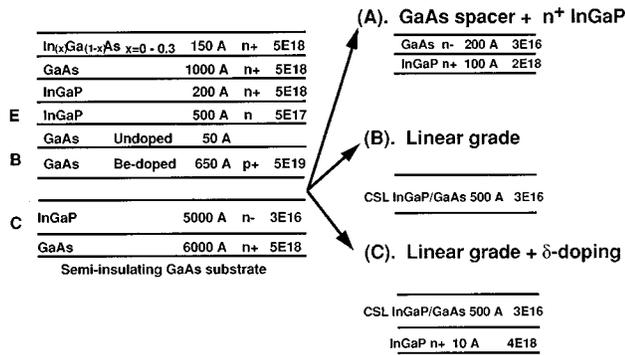
FIG. 1. Structures of devices A, B, and C.
