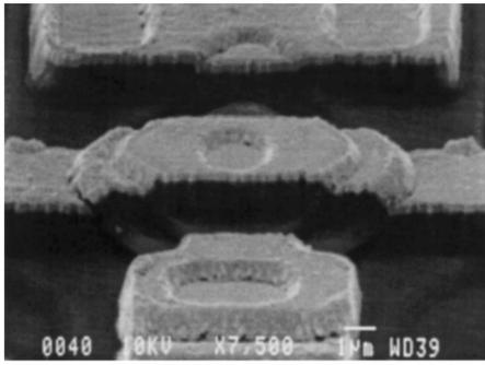
FIG. 3. Scanning electron microscopy (SEM) pictures of a  $32 \mu\text{m}^2$  device. The base and emitter are aligned along (010) and (001) planes.
