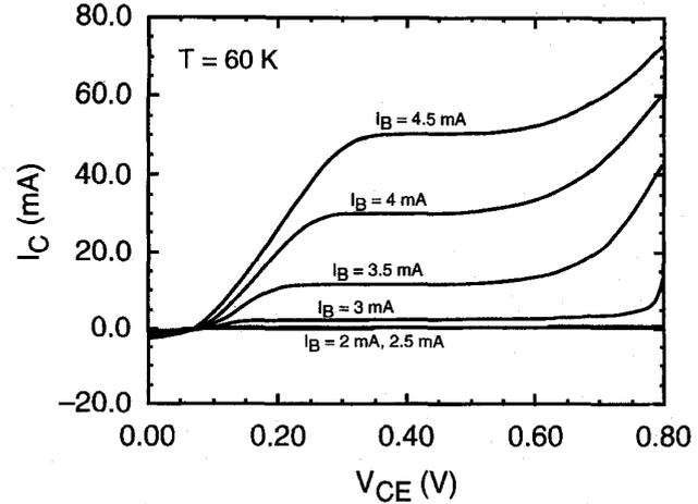
Fig. 3. InAs transistor common-emitter characteristics at 60 K. The base currents are 2 mA to 4.5 mA in 0.5 mA steps, and the device size is  $24 \times 24 \mu\text{m}^2$ .
