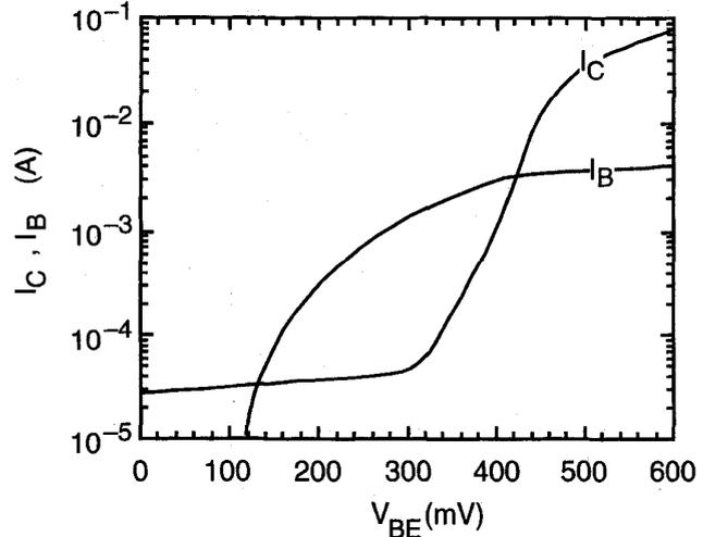
Fig. 4. Gummel plot of  $24 \times 24 \mu\text{m}^2$  InAs transistor at  $T = 30 \text{ K}$ . The base-collector junction reverse bias is 150 mV.
