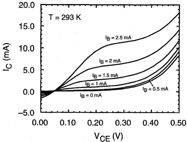
Fig. 2. InAs transistor common-emitter characteristics at room temperature. Base currents are 0 to 2.5 mA in 0.5 mA steps and the emitter size is  $24 \times 24 \mu\text{m}^2$ .
