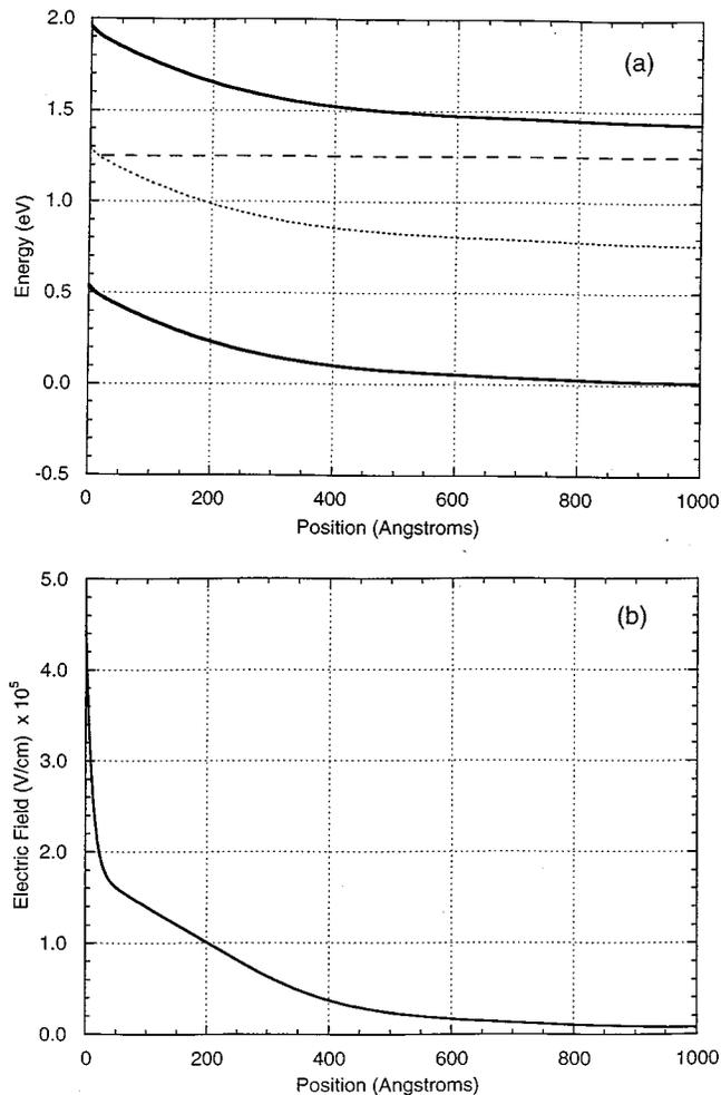
FIG. 3. Self-consistent Poisson's calculation of (a) the band profile and (b) the magnitude of the field distribution  $E(z)$  as a function of position from the surface for LTG:GaAs for (a) a trap density ( $N_T$ ) of  $1 \times 10^{20} \text{ cm}^{-3}$  having a Gaussian distribution of states with width  $\sigma (= 0.2 \text{ eV})$ , the peak of the Gaussian distribution occurring 0.25 eV below the intrinsic Fermi level and (b) midgap surface Fermi level pinning.
