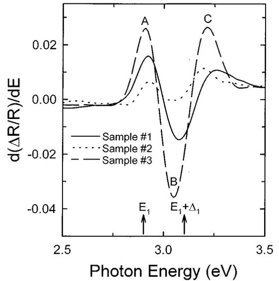
FIG. 2.  $d(\Delta R/R)/dE$  spectra of sample Nos. 1 (solid line), 2 (dotted line), and 3 (dashed line). The positions of the  $E_1$ ,  $E_1 + \Delta_1$  features are denoted by arrows at the bottom of the figure.
