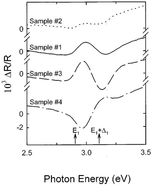
FIG. 1. RAS spectra of sample Nos. 1 (solid line), 2 (dotted line), 3 (dashed line), and 4 (dot-dashed line). The positions of the  $E_1$ ,  $E_1 + \Delta_1$  features are denoted by arrows at the bottom of the figure.
