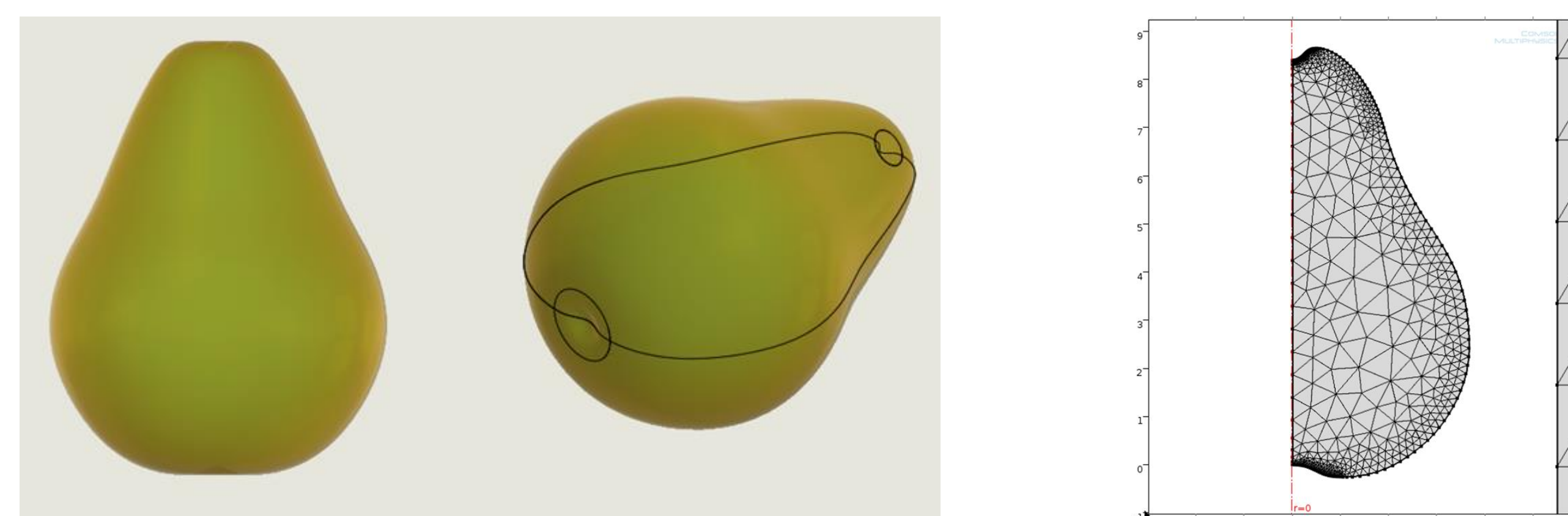
Mesh details on the geometric domain
