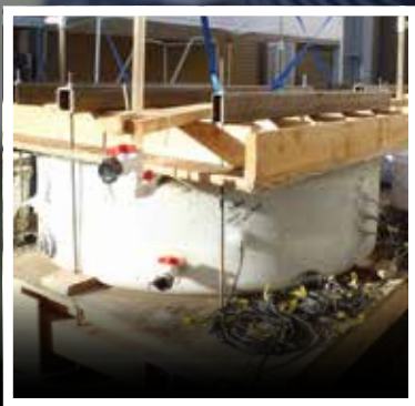
Main image: bio-cemented soil. Inset: Biocementation treatment in 2-m-diameter tanks: Figure 1a . Setup.
