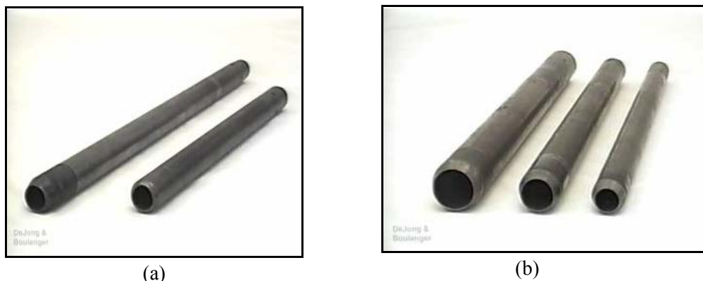
Figure 3-7: Split-Barrel Samplers: (a) Lengths of 457 mm (18 in) and 610 mm (24 in); (b) Inside diameters from 38.1 mm (1.5 in) to 89 mm (3.5 in).
