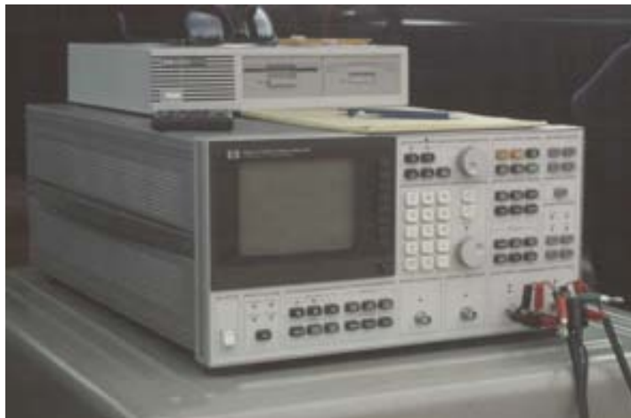
Figure 5-29. Spectrum Analyzer and Data Logging Equipment for SASW.
