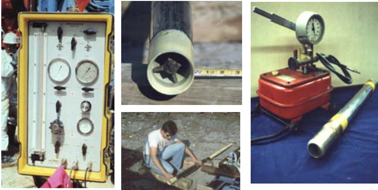
Figure 5.18. Photos of Pressuremeter Equipment, including Menard-type pressure panel, SBP probe, SBP cutter teeth, hydraulic jack, and monocell-type probe.
