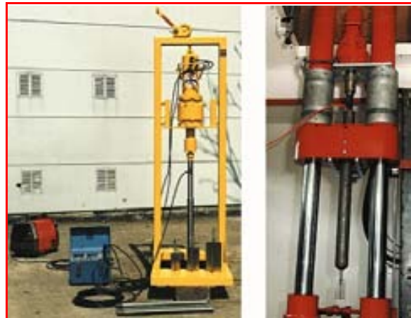
Figure 5-10. Selection of Vane Shear Blades, Pushing Frames, and Torquemeter Devices.
