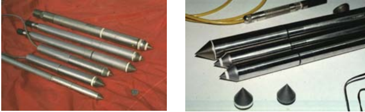
Figure 5-5. Various Cone Penetrometers Including Electric Friction and Piezocone Types.
