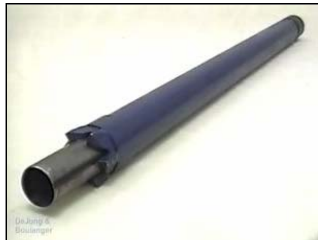
Figure 3-14: Pitcher Tube Sampler.
