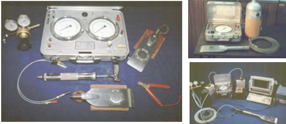
Figure 5-15. Flat Plate Dilatometer Equipment: (a) Modern Dual-Element Gauge System; (b) Early Single-Gauge Readout; (c) Computerized Data Acquisition Model.
