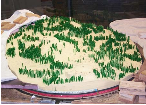
Figure 3: Wind Tunnel Scaled Model of the Berkeley Hills with the Lawrence Berkeley National Laboratory.
