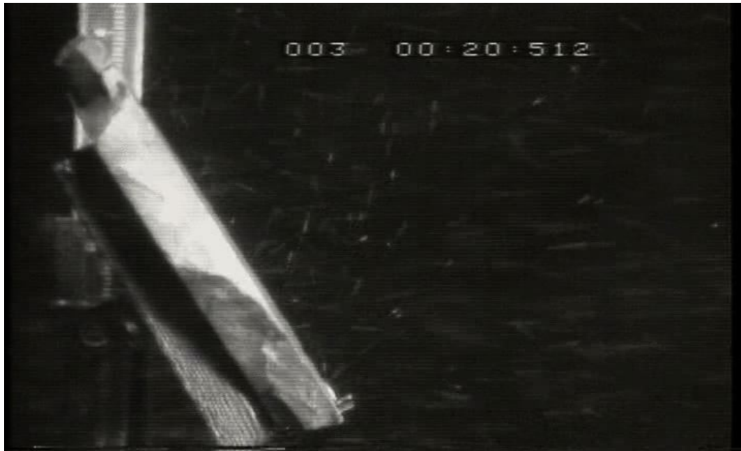
Figure 4. Basaltic rock at 60° with tunnel speed at 11 m/s at terrestrial pressure.
