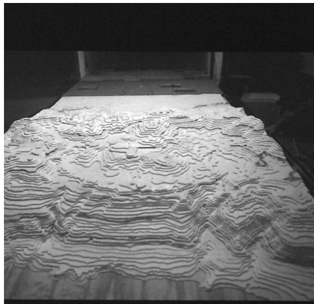
Figure - 2. The scaled (1:5,000) model of the site placed in the wind-tunnel.
