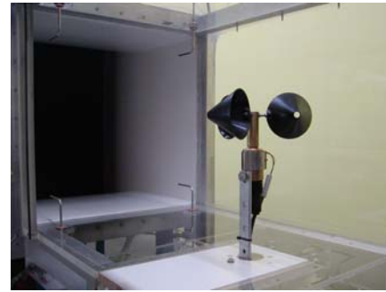
Figure 6: Anemometer calibration testing using a Pitot-static tube system.
