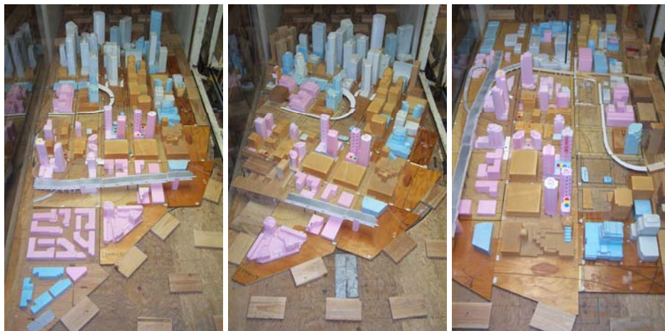
Figure 12. Folsom and Main East and West buildings, northwest, west-northwest and southwest wind directions, shown left-to-right, for the existing setting (winds blow from top to bottom).
