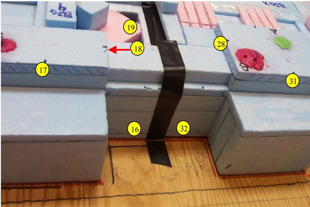
**Figure 5.** Receptor locations in model, picture taken of the East side of the Building Nos. 3 and 4.
