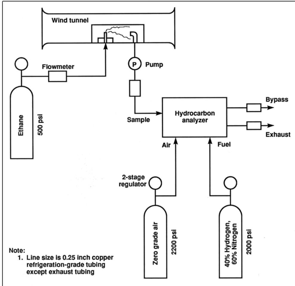
Figure B-1: Schematic diagram of gas dispersion concentration measurement system.
