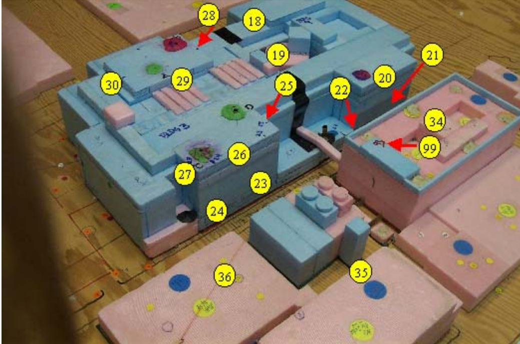
**Figure 4.** Receptor locations on model, picture taken of the West side of Building Nos. 3 and 4.
