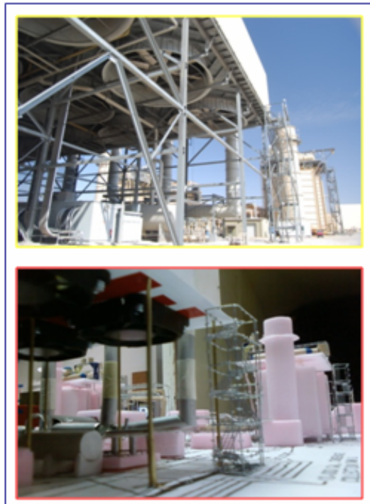
Figure 9 Verification of Model Geometry by Comparison with Full Scale
