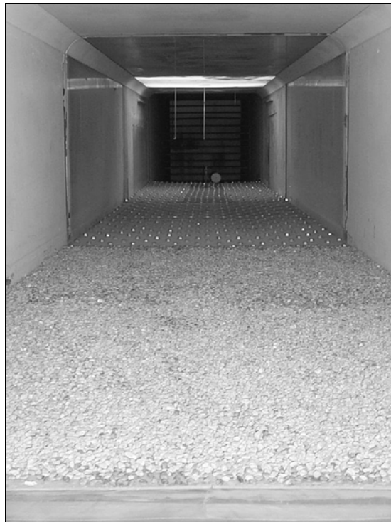
Figure 3.12: Downwind photo of MARSWIT displaying pebble boundary-layer trip.
