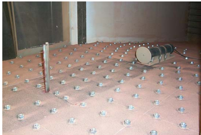
Figure 4.56: Photo of Test Bed 3 after a dust threshold experiment at bulk Ri \approx -0.0012 unstable boundary layer conditions.
