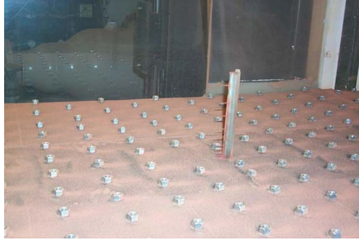
Figure 4.55: Photo of Test Bed 3 after a dust threshold experiment at bulk Ri \approx 0 neutral boundary layer conditions.
