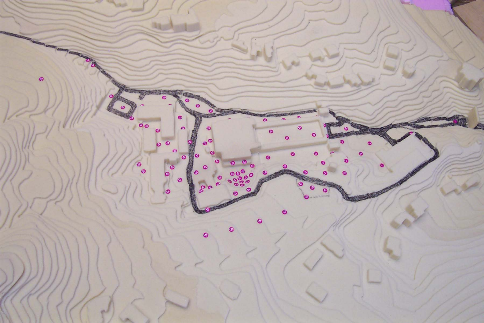
Figure 6. Photograph of the wind-tunnel model of the Getty Villa site, scale is one inch equal 75 feet.
