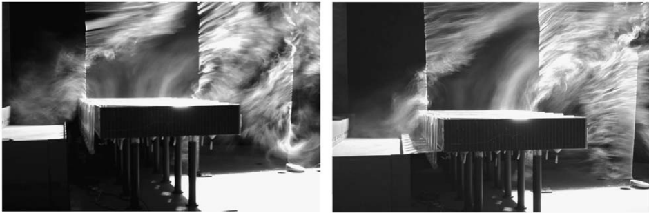
Fig. 5. Flow visualization for Models 1 and 4 (with additional platform between the top of steam turbine room and the platform of condensers platform) at \beta = 0^\circ .
