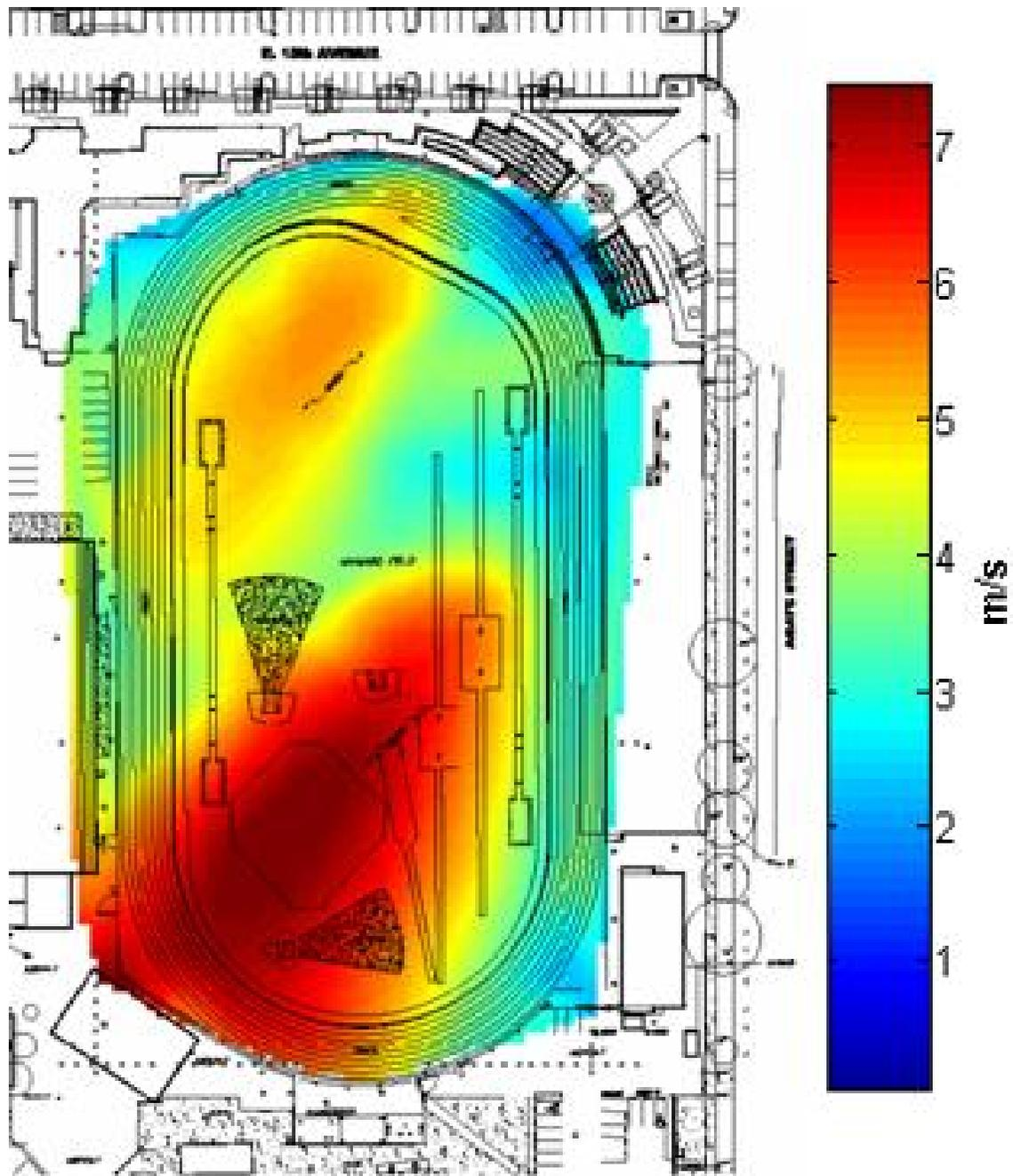
**Figure 7.** Predicted full-scale pedestrian-level (5 feet or 1.5 meters above ground level) wind speeds are shown for a northeast oncoming wind without wind screen protection. The reference velocity is assumed to be 7.5 m/s at a reference height of 10 m. The highest wind speeds exist in the southwest corner, which reach or exceed 7.5 m/s.
