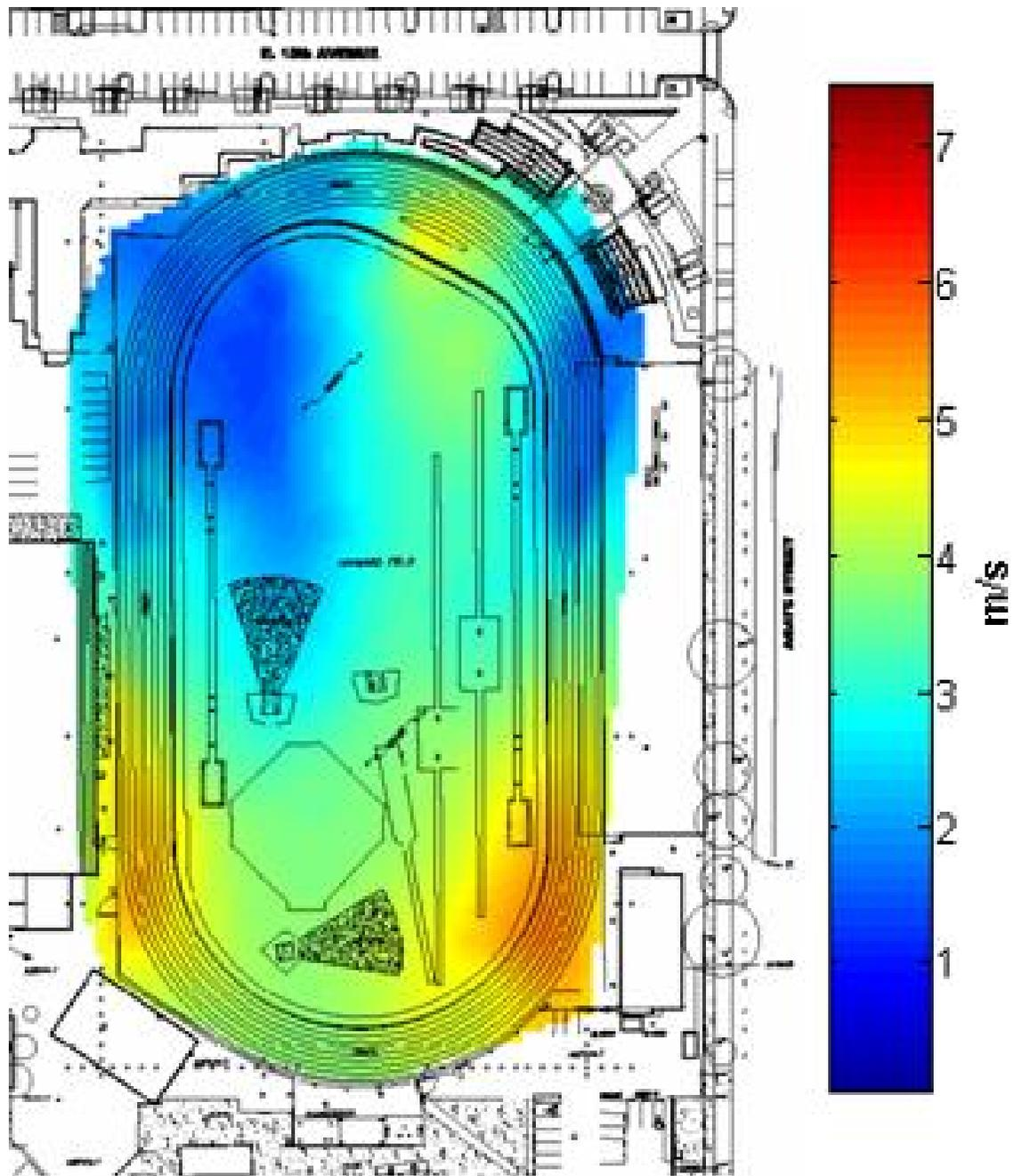
**Figure 4.** Predicted full-scale pedestrian level (5 feet or 1.5 meters above ground level) wind speeds are shown for a north oncoming wind with wind screen protection. All wind screens are positioned 90 degrees counter-clockwise from the north. The reference velocity is assumed to be 7.5 m/s at a reference height of 10 m. The results show reduction in the northwest corner below 2 m/s. There are three regions where the wind speed nearly reaches or exceeds 5 m/s.
