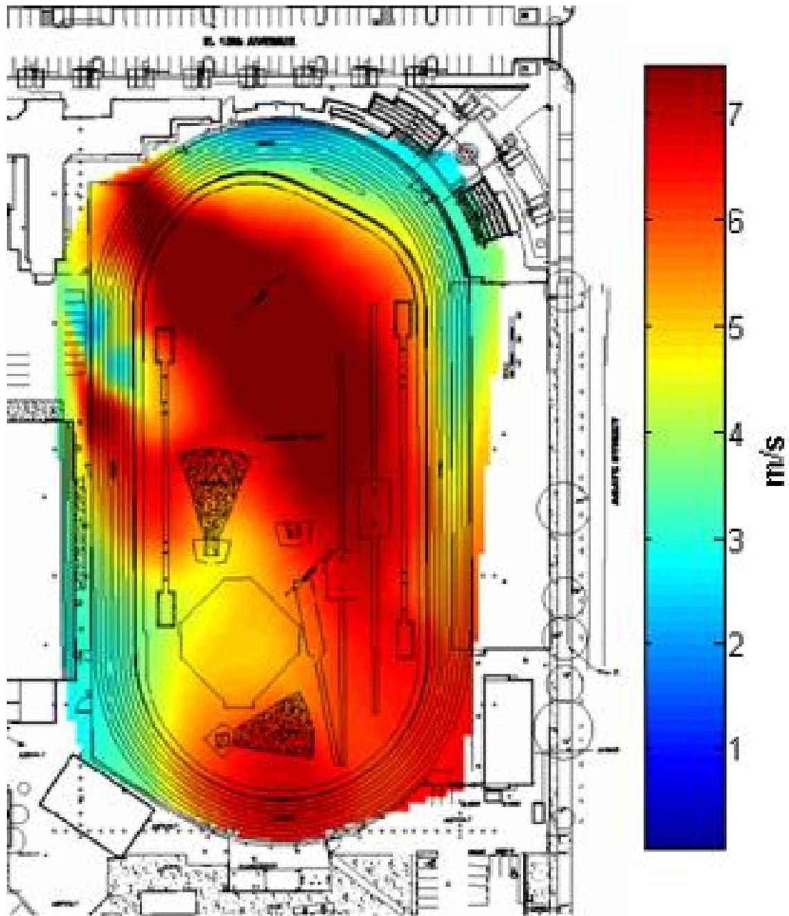
**Figure 11.** Predicted full-scale pedestrian level (5 feet or 1.5 meters above ground level) wind speeds are shown for a northwest oncoming wind without wind screen protection. The reference velocity is assumed to be 7.5 m/s at a reference height of 10 m. The highest wind speeds, which reach or exceed 7.5 m/s, exist in the northern region of the field.
