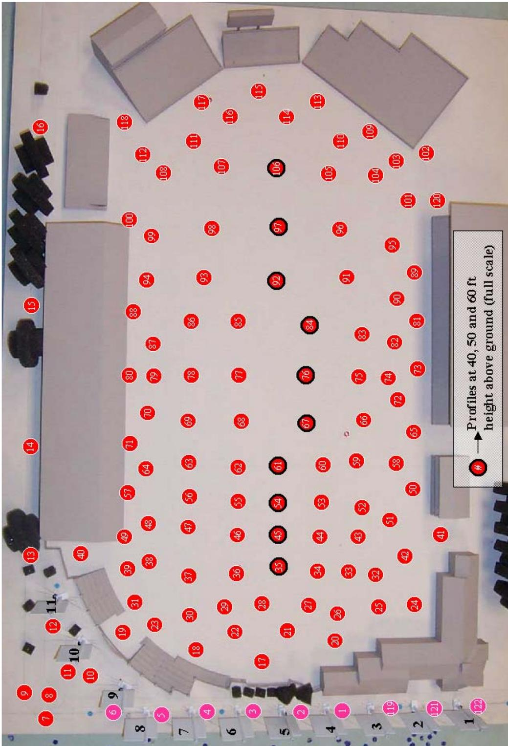
**Figure 2.** Measurement locations on wind-tunnel model, note north is down.
