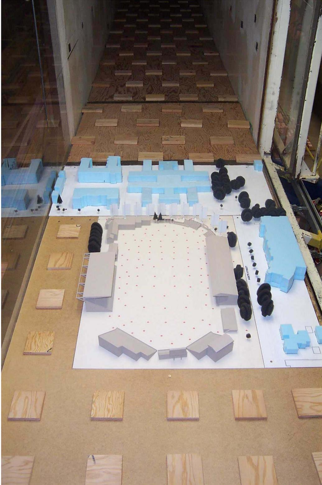
**Figure 1.** Wind-tunnel model in wind tunnel, simulating a north wind with the eleven pylons (screens) at 90 degrees to oncoming wind.
