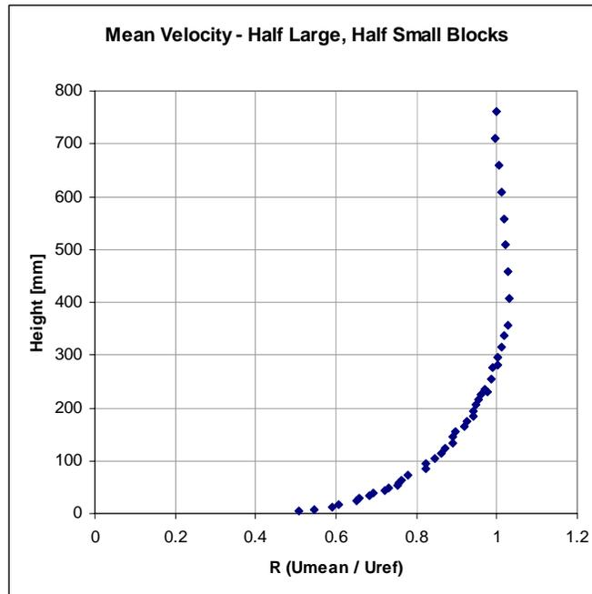
**Figure D-1.** Mean velocity profile in terms of  $R$  ( $U_{\text{mean}}/U_{\text{ref}}$ ) for a typical wind direction in the wind tunnel. The power law exponent  $\alpha$  is approximately 0.2. The reference velocity is 3.16 m/s.
