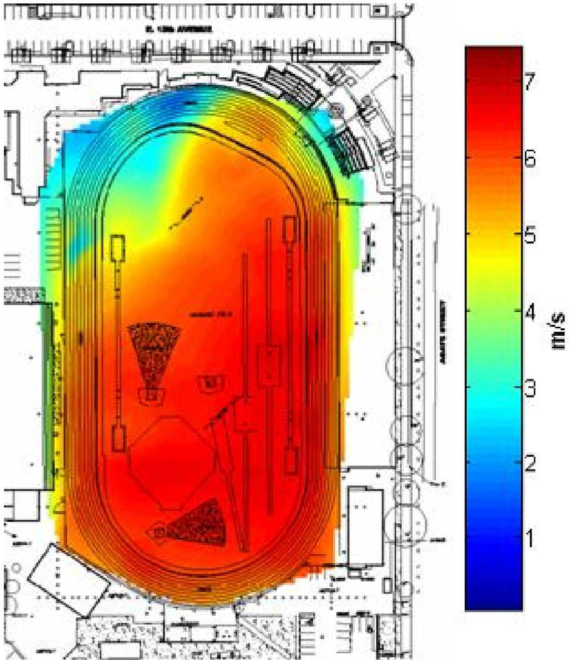
**Figure 3.** Predicted full-scale pedestrian level (5 feet or 1.5 meters above ground level) wind speeds are shown for a north oncoming wind without wind screen protection. The reference velocity is assumed to be 7.5 m/s at a reference height of 10 m. The results show that the field is dominated by wind speeds in excess of 6 m/s.
