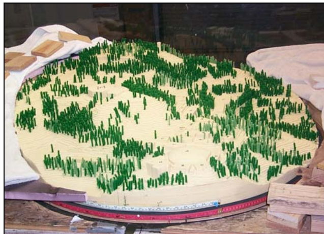
Figure 3: Wind tunnel scaled model of the Berkeley hills with the Lawrence Berkeley National Laboratory.
