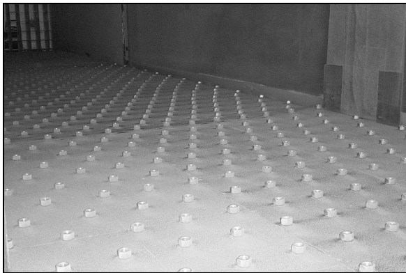
Figure 3.24: Upwind view of test bed and immediate fetch for second roughness condition.
