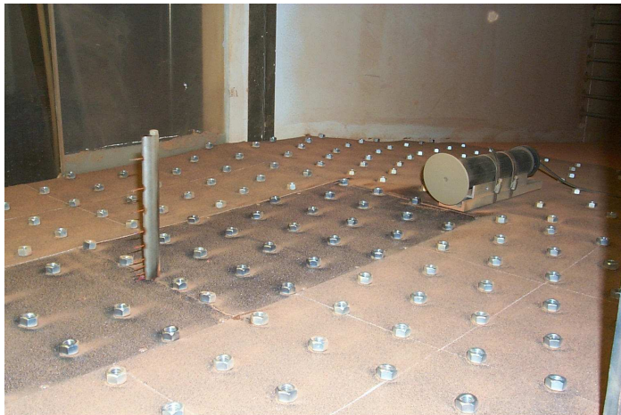
Figure 4.57: Photo of Test Bed 3 after a dust threshold experiment at bulk Ri \approx -0.0024 unstable boundary layer conditions.
