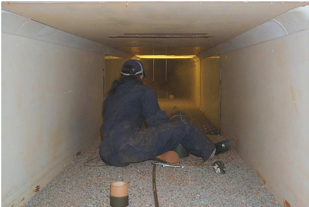
Figure 3.19: Photo of experimenter prepping the dust suspension system just at the end of the pebble-bed boundary layer trip.
