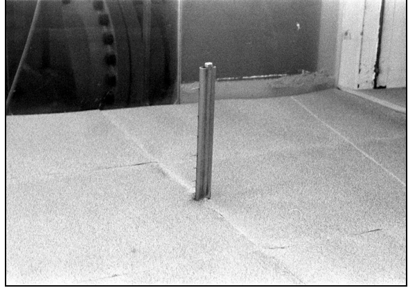
Figure 3.22: Test section view of first roughness configuration.
