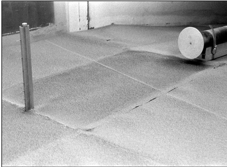
Figure 3.15: Photo of electrometer probe situated at the end of the test section and slightly offset from the thermocouple rake.
