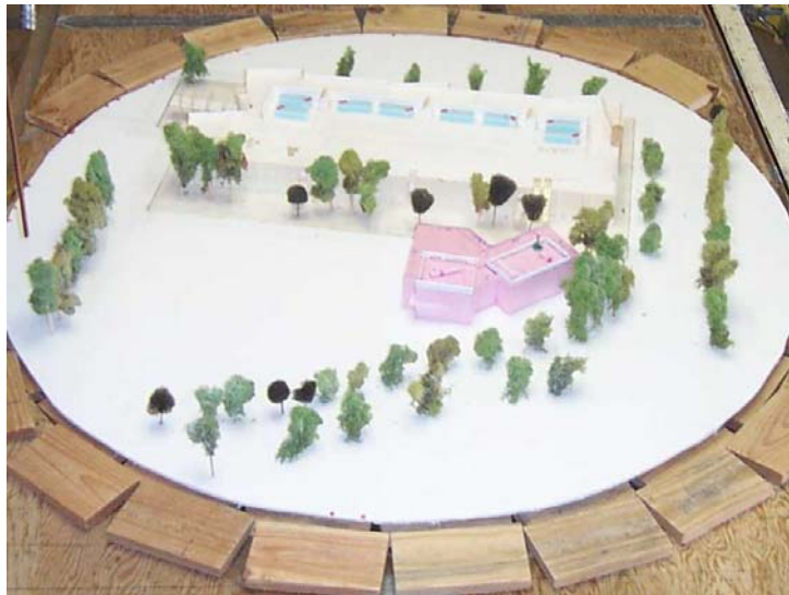
Figure 1: Wind tunnel turntable model of UC Davis Watershed Science Research Center.
