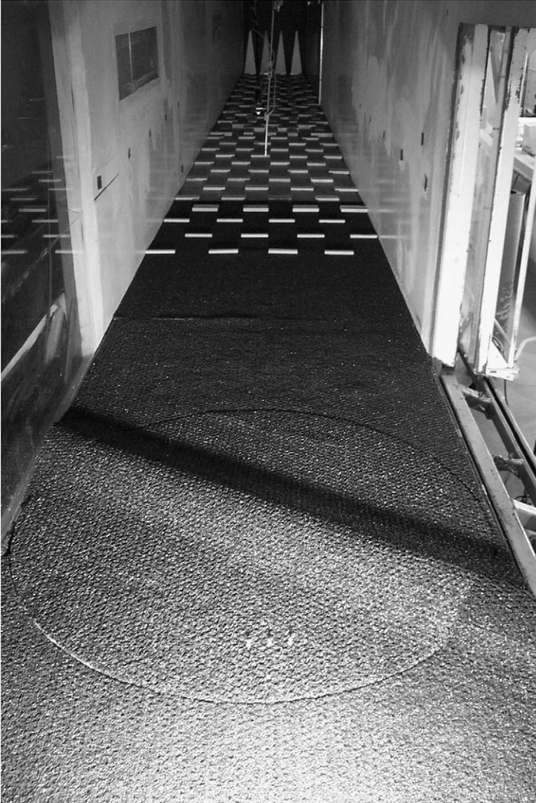
Fig. 2. Roughness element arrangement used in ABLWT development section for generalized hill tests. Also visible is the two-dimensional hill model at  $\theta = 30^\circ$  and the measurement probe support with sighting laser and height probe installed.
