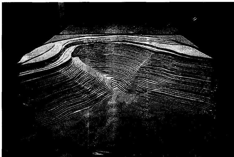
Fig. 5. Photograph of climbing dune wind-tunnel model.
