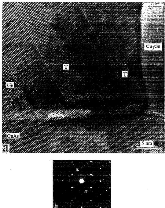
FIG. 2. (a) High-resolution TEM image showing the interface between a large epitaxial Ge grain and the GaAs substrate. Typical twin lamella are denoted by T. Arrow indicates an amorphous pocket at the interface. (b) Corresponding SAD pattern showing the [110] zone axis pattern of GaAs and Ge (unresolved) with typical twin spots (denoted by T).
