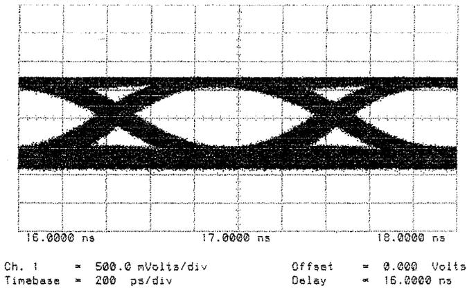
Fig. 2. Eye diagram for  $2^{31} - 1$  PRBS at 1 Gb/s.
