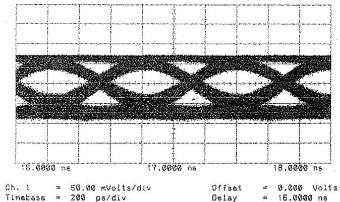
Fig. 3. Eye diagram for  $2^{31} - 1$  PRBS at 1.7 Gb/s.
