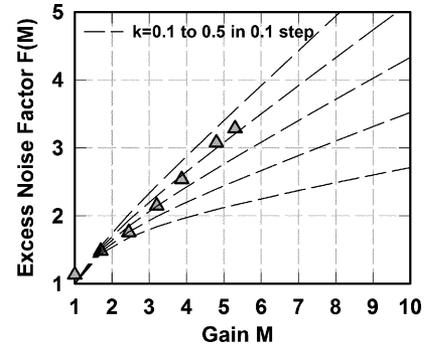
Fig. 4. Excess noise factor versus gain for the standard GaP APD: UV(351, 363 nm), RT.
