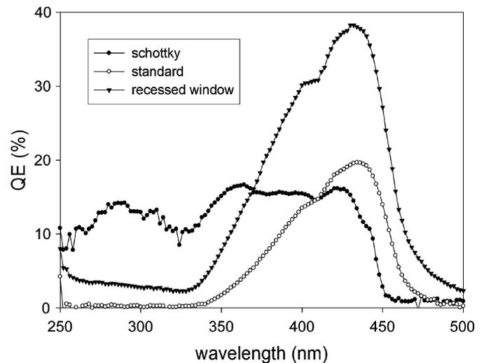
Fig. 3. QE of a standard GaP APD, a recessed window GaP APD, and a Schottky photodiode, measured at unity gain.
