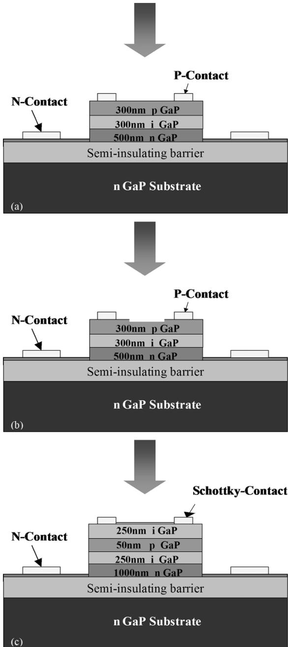
Fig. 1. Cross section of GaP APD. (a) Standard. (b) Recessed window APD. (c) Schottky.
