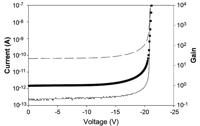
Fig. 2.  $I$ – $V$  characteristic for an  $80 \mu\text{m}$  diameter device.  $I$ – $V$  curves were the same for both standard and recessed window APDs.
