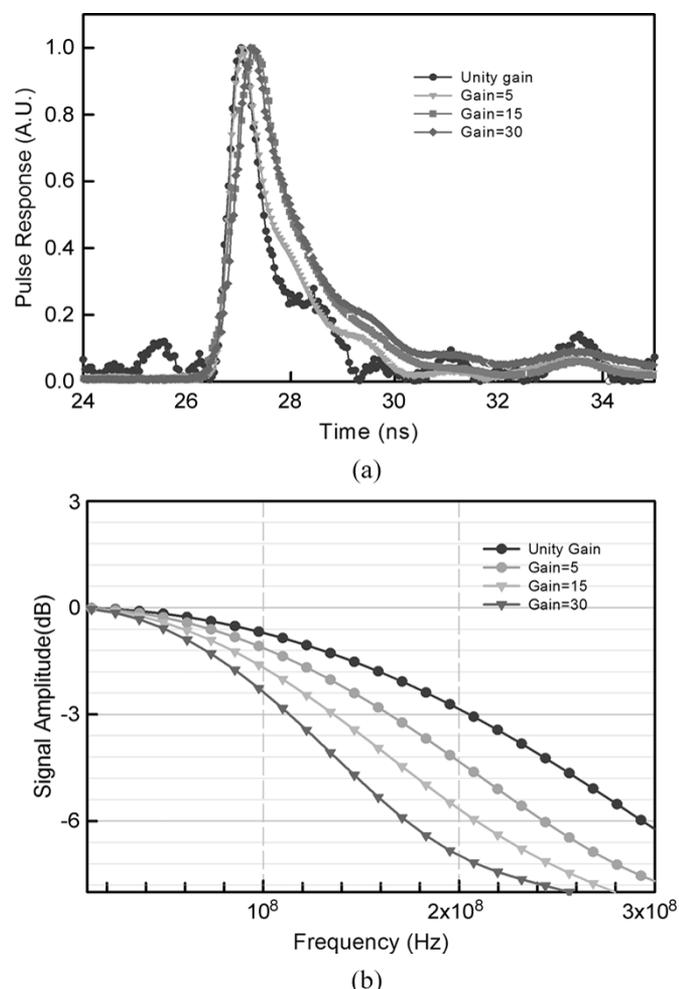
Fig. 5. (a) Normalized time domain speed response. (b) Bandwidth of GaP APDs.
