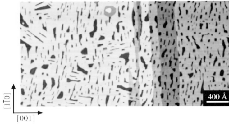
Figure 2. Topography image of a 20 Å thick Bi film grown at T = 140 K on InP(110). V_{bias} = 250 mV, I_T = 100 pA, field of view: 3900 \text{ \AA} \times 1950 \text{ \AA} .
