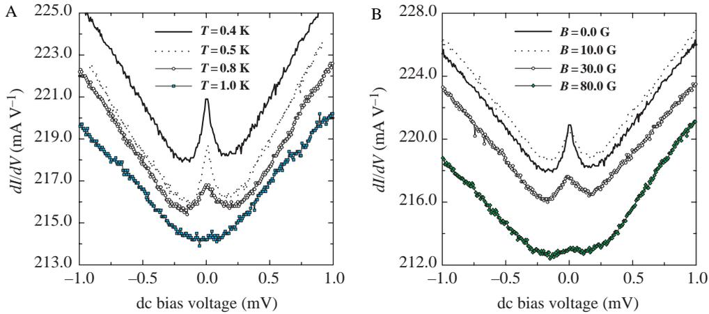
**Fig. 6.** Conductance versus the dc bias voltage for Sample 3 for A, different temperatures, and B, different magnetic fields. A conductance peak develops near zero bias voltage, a correction to Giaever tunneling arising from weak localization inside the normal metal.
