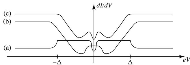
**Fig. 8.** Possible explanation for conductance dip around zero voltage observed inside the zero bias conductance peak. Low transmission regions of the interface give both the overall Giaever tunneling shape of the  $dI/dV$  versus  $V$  and the zero bias conductance peak. A few high transmission regions of the contact could produce the zero bias conductance dip.
