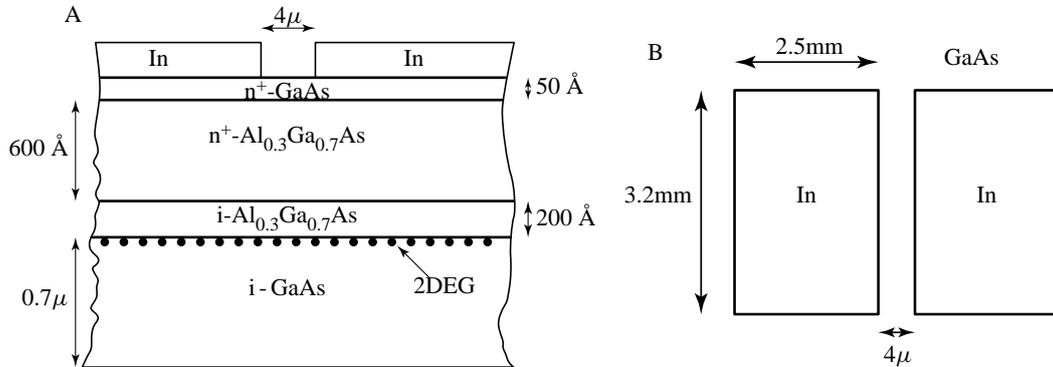
**Fig. 2.** A, Cross-section of the AlGaAs/GaAs heterostructure before annealing the superconducting In contacts. B, Top view of the contact geometry.
