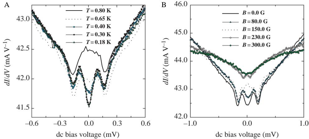
**Fig. 7.** Conductance versus the dc bias voltage for Sample 4 for A, different temperatures, and B, different magnetic fields. The additional conductance dip which develops around zero bias voltage can be explained by an inhomogeneous NS contact consisting of both high and low transmission regions.
