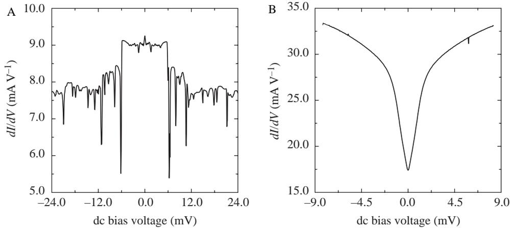
**Fig. 5.** Conductance versus the dc bias voltage across the two Indium pads for A, Sample 1 and B, Sample 2. Sample 1 shows nearly 100% ballistic transport of electrons (after correcting for series resistance), while Sample 2 shows Giaever tunneling (through a tunnel barrier having transmission of the order  $T \simeq 0.1$ ).
