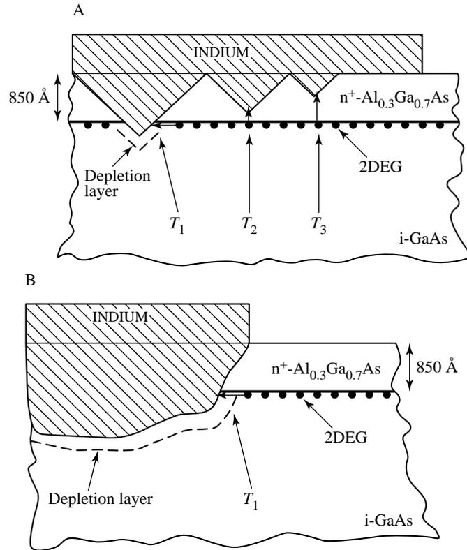
**Fig. 1.** Schematic of the In profile obtained after annealing for A, low temperature/short time anneal (Sample 1), and B, a higher temperature/longer time anneal (Sample 2). Penetration of In into the AlGaAs layer is guided along a preferred crystallographic direction in A, forming point contacts to the 2DEG. The point contacts grow together and penetrate the 2DEG in B.
