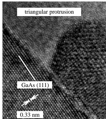
**Fig. 4.** High magnification TEM photograph of a portion of a single In point contact grown into a (100) AlGaAs surface. In growth into the AlGaAs is strongly guided along the {111} planes.
