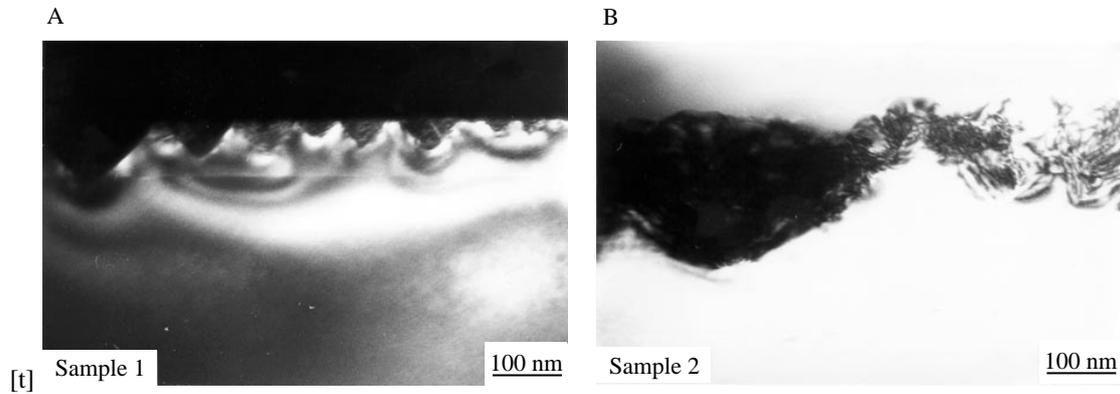
**Fig. 3.** TEM photographs of an In-AlGaAs/GaAs contact annealed A, for a short time (Sample 1) and B, a longer time (Sample 2). Penetration of In into the sample is guided by the {111} planes, forming the In point contacts which are clearly observable in A. The point contacts agglomerate and grow through the AlGaAs/GaAs interface in B.
