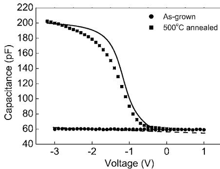
FIG. 2. Measured capacitance-voltage ( $C$ - $V$ ) characteristics of as-grown (circle symbols) and annealed (square symbols) GaAs MIS capacitors, with the simulated results (the solid line for ideal MIS and the dashed line for MIS with  $D_s = 3 \times 10^{13} \text{ cm}^{-2}$ ).
