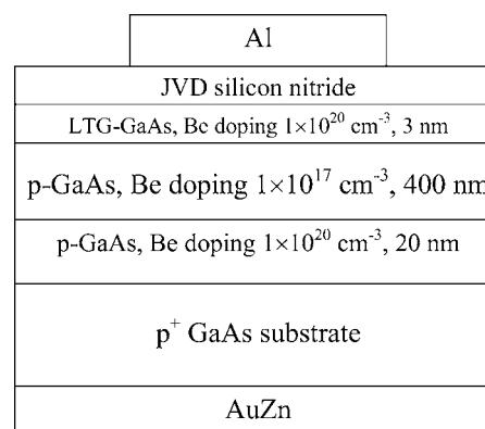
FIG. 1. Structure of the Al/SiN/GaAs MIS capacitor.
