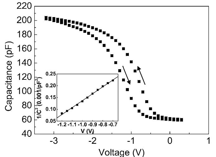
FIG. 3. Measured capacitance-voltage ( $C$ - $V$ ) hysteresis of the Al/SiN/GaAs MIS capacitor. The inset shows the  $1/C^2 \sim V$  fitting in the depletion region.
