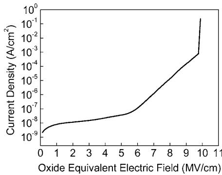
FIG. 4. Measured current-voltage (*I*-*V*) characteristics of the Al/SiN/GaAs MIS capacitor.
