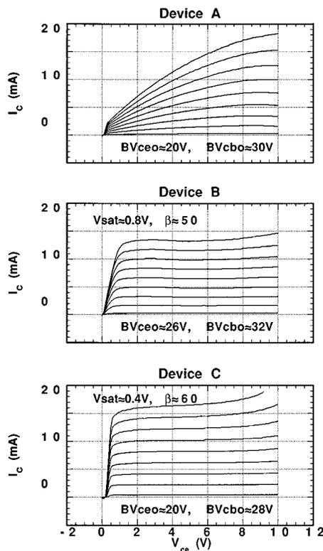
FIG. 4. dc characteristics of devices A, B, and C.
