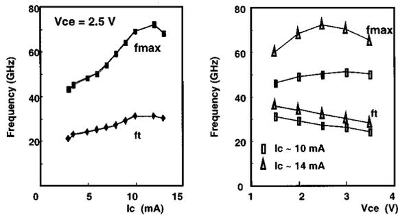
FIG. 6. Cutoff frequency ( $f_t$ ) and maximum oscillation frequency ( $f_{\max}$ ) of a  $32 \mu\text{m}^2$  device at different bias conditions.
