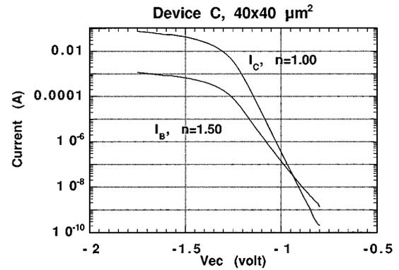
FIG. 5. Gummel plot of a large-area ( $40 \times 40 \mu\text{m}^2$ ) device C.
