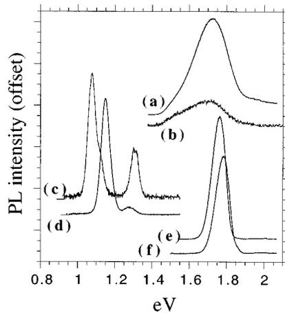
FIG. 3. PL at 77 K (a) from InAs/GaP QDs at 77 K and (b) at 300 K. (c), (d) From low surface densities of InGaAs/GaAs quantum dots. Wetting layer luminescence is shown on both spectra. (e) and (f) PL intensity from AlInAs/AlGaAs quantum dots shown for comparison (77 K).
