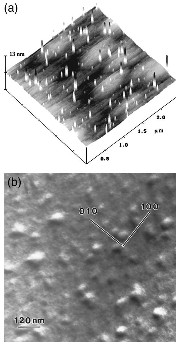
FIG. 2. (a) Surface FM plot of InAs islands on GaP showing broad size distribution. Vertical enhancement:  $Z=28(X,Y)$ . Micron scale undulations are seen on the surface of GaP for many of the growths independently of InAs island formation. (b) Plan view TEM micrograph of InAs dots in a GaP matrix.
