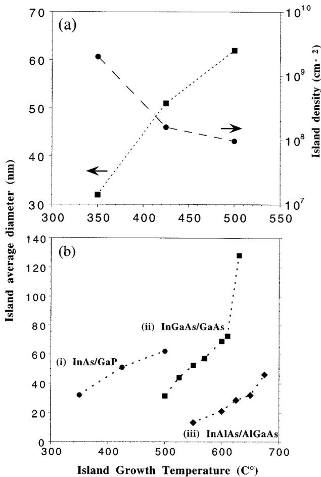
FIG. 1. (a) Temperature dependence of average sizes and concentrations in InAs islands self-formed on GaP surfaces. Values were obtained from statistical analysis of FM images. (b) Comparison of island diameters obtained for (i) InAs/GaP V-W QDs and for S-K type QDs, (ii) InGaAs/GaAs, and (iii) AlInAs/AlGaAs.
