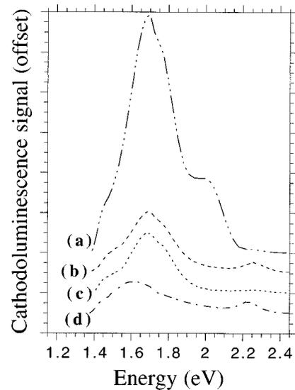
FIG. 4. CL spectra from capped InAs islands grown on GaP. (a) 15 keV electron beam accelerating voltage at a sample temperature of 8 K. (b), (c) 300 K and plan view excitation at 20 and 15 keV, respectively. (d) Edge excitation of a cleaved sample away from the surface. 20 keV and 300 K.
