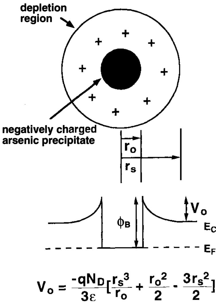
Figure 14 Schottky barrier model for the embedded arsenic precipitates.
