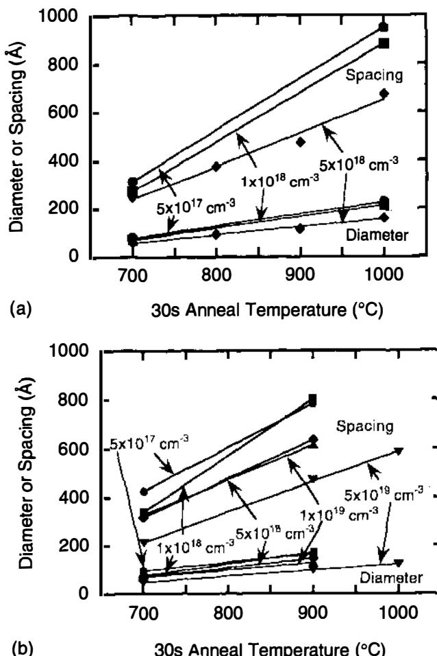
**Figure 16** Average cluster sizes and spacings as a function of anneal temperature for 30-s isochronal annealing of LTG-GaAs epilayers for (a) three different Si-doping levels and (b) five different Be-doping levels.
