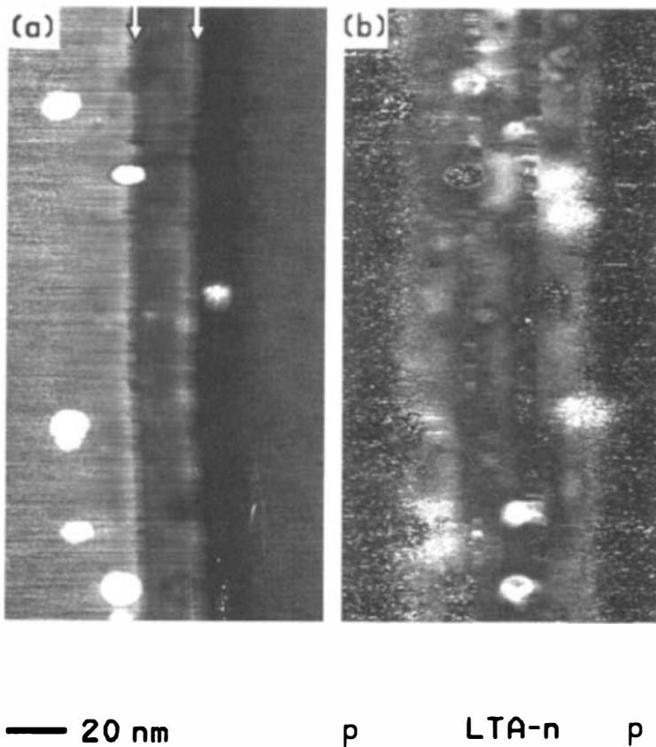
**Figure 24** STM image of a cleaved GaAs structure, showing (a) topography and (b) conductance, acquired at a sample voltage of  $-2.5 \text{ V}$ . The gray-scale range in (a) is 8 Å. As indicated in (b), the structure contains an LTA *n*-type layer, surrounded by *p*-type layers grown at higher temperature. The sample was annealed at 600°C. Two steps occur in the LTA-layer, as marked by arrows in (a).
