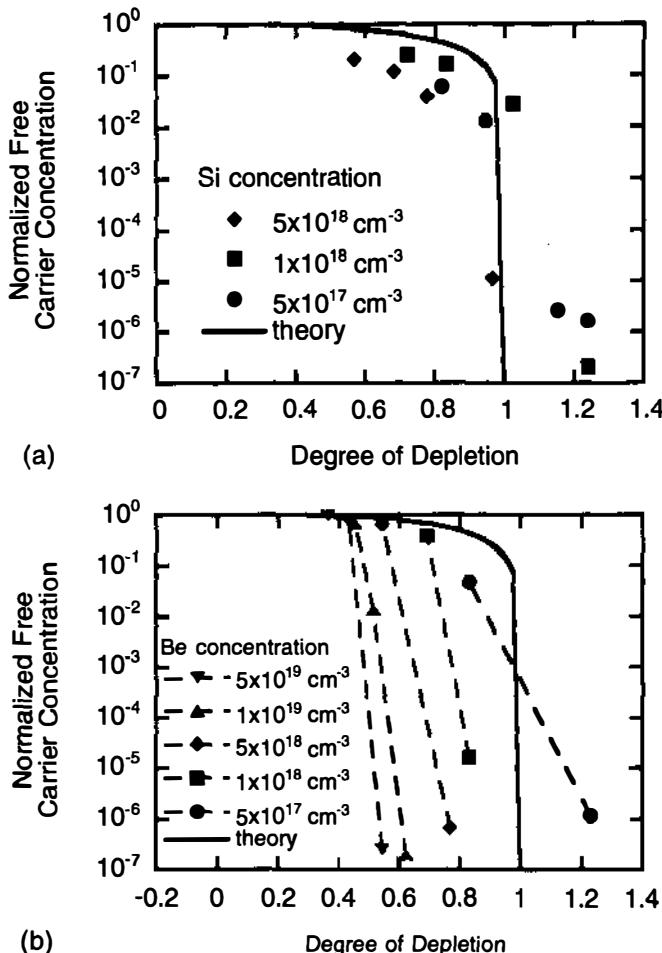
Figure 15 Normalized carrier concentration vs degree of depletion for (a) three different Si-doping levels and (b) five different Be-doping levels. Degree of depletion is  $2 r_s/d$ , where  $r_s$  is the depletion sphere radius and  $d$  is the distance between precipitates.
