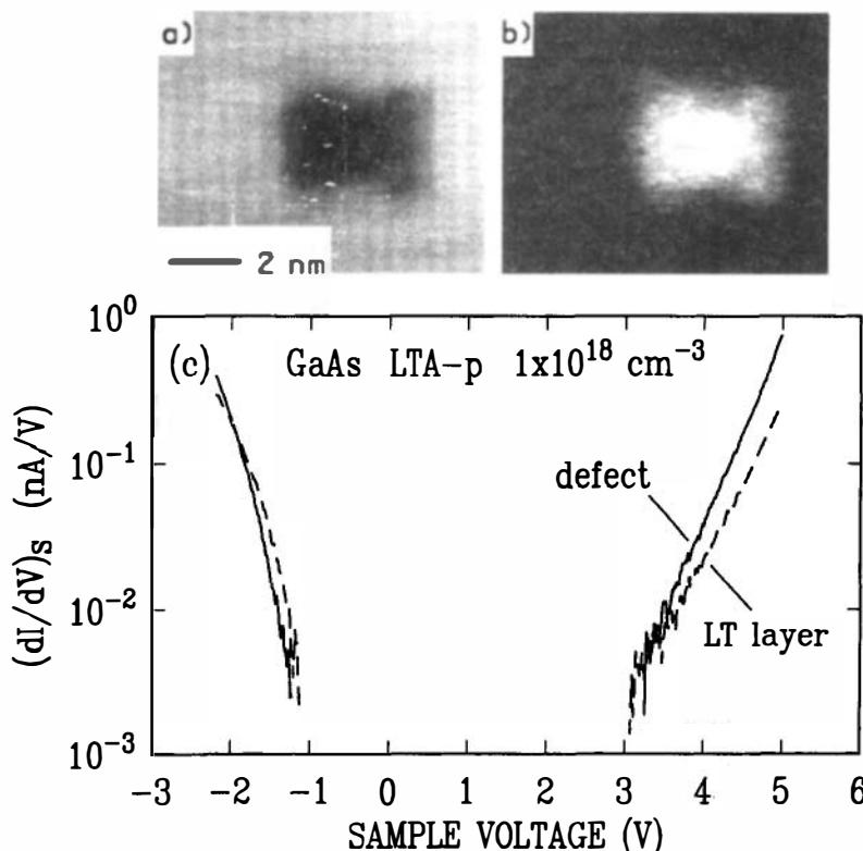
**Figure 29** STM image of same sample as in Figure 28, displaying an expanded view of a point defect (arsenic antisite). Image (a) shows topography and (b) conductance, acquired at a sample voltage of  $-2.2$  V. The gray-scale range in (a) is  $1.1$  Å. Tunneling spectra are shown in (c), acquired on the point defect and on a region of flat LTA-GaAs between defects.
