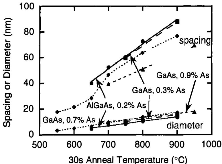
**Figure 3** Density and average size of arsenic clusters in four different epilayers as a function of temperature for a 30 s anneal. Three of the epilayers are GaAs, one containing 0.3% excess arsenic, one containing 0.7% excess arsenic, and one with 0.9% excess arsenic. The fourth epilayer is AlGaAs containing 0.2% excess arsenic.
