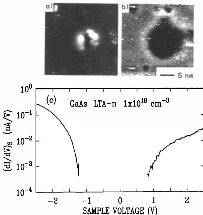
**Figure 27** STM image of LTA *n*-type layer, showing (a) topography and (b) conductance, acquired at a sample voltage of  $-2.5$  V. The gray-scale range in (a) is  $2.0$  Å. The sample was annealed at  $700^\circ\text{C}$ . A tunneling spectrum (conductance at constant tip-sample separation) is shown in (c), acquired on a flat region of LTA-GaAs between precipitates.
