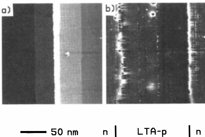
Figure 28 STM image of a cleaved GaAs structure, showing (a) topography and (b) conductance, acquired at a sample voltage of  $-2.2 \text{ V}$ . The gray-scale range in (a) is 22 Å. As indicated in (b), the structure contains an LTA *p*-type layer, surrounded by *n*-type layers grown at higher temperature. The sample was annealed at  $700^\circ\text{C}$ . Several steps occur in the LTA-layer, as seen in (a).
