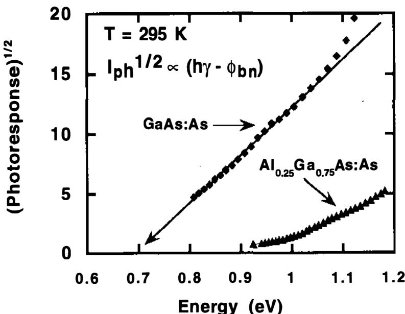
Figure 32 Photoresponse vs photon energy for two *PiN* diodes. One *p-i-n* diode has an *i*-layer of GaAs containing arsenic clusters, and the other has an *i*-layer of  $\text{Al}_{0.25}\text{Ga}_{0.75}\text{As}$  containing arsenic clusters. The *p*- and *n*-regions are normal highly stoichiometric material.
