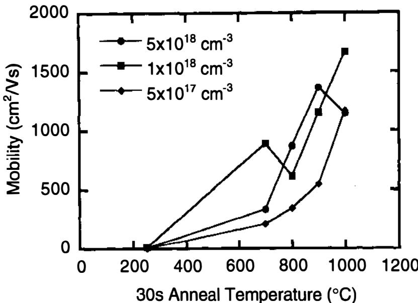
Figure 13 Mobility as a function of anneal temperature for 30-s isochronal anneals for the Si-doped LTG-GaAs epilayers.
