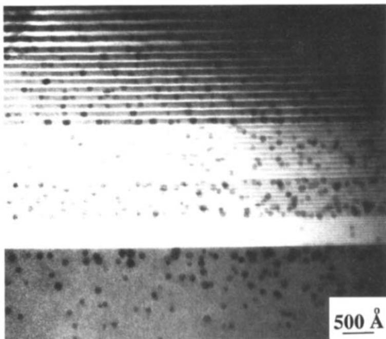
Figure 7 A series of 10-period superlattices of progressively wider  $\text{Al}_{0.3}\text{Ga}_{0.7}\text{As}$  barriers or GaAs wells grown at low temperatures and then annealed at 700°C for 30 s.
