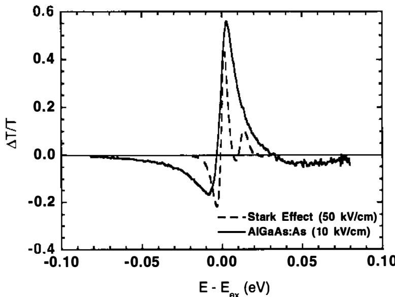
Figure 36 Comparison of the quantum-confined Stark effect in a high-quality, highly stoichiometric multiple-quantum well structure and in an AlGaAs epilayer containing arsenic clusters.
