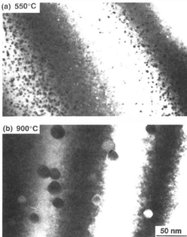
Figure 2 TEM images of two samples from the same LTG-GaAs epilayer that were annealed at (a) 550°C for 30 s and (b) 900°C for 30 s.
