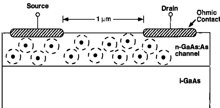
Figure 33 Cross section of metal-semiconductor-metal photoconductor showing depletion regions surrounding the arsenic precipitates in the channel.
