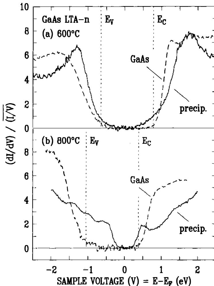
Figure 26 STM spectra acquired from LTA *n*-type layers, annealed at (a) 600°C and (b) 800°C. Spectra are shown acquired on the arsenic precipitates (solid line) and on regions of bare LTA GaAs in between the precipitates (dashed line). The valence and conduction band edges are marked by  $E_V$  and  $E_C$  respectively.
