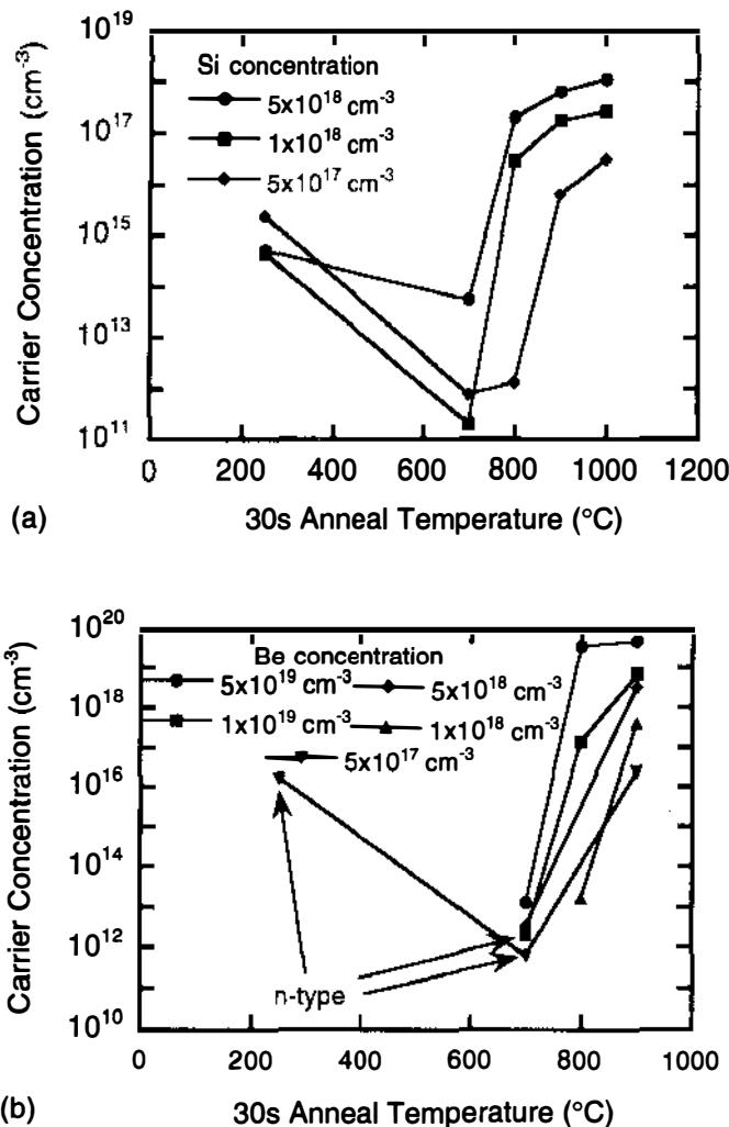
**Figure 12** Carrier concentration as a function of temperature for 30-s isochronal annealing of GaAs epilayers containing excess arsenic for (a) three different *n*-type doping concentrations and (b) five different *p*-type doping concentrations.
