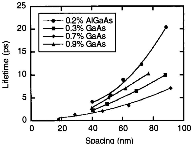
**Figure 31** Carrier lifetime vs cluster spacing, fit by a square dependence on cluster spacing for four epilayers. Three of the epilayers are GaAs, one containing 0.3% excess arsenic, one containing 0.7% excess arsenic, and one with 0.9% excess arsenic. The fourth epilayer is AlGaAs containing 0.2% excess arsenic.
