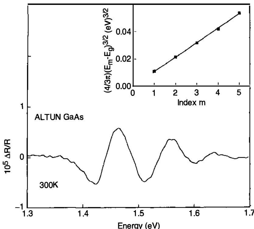
**Figure 18** Contactless electroreflectance spectrum from the ALTUN structure at 300 K. The inset shows a plot of  $(4/3\pi)(E_m - E_g)^{3/2}$  as a function of the Franz-Keldysh oscillations extrema index  $m$ .
