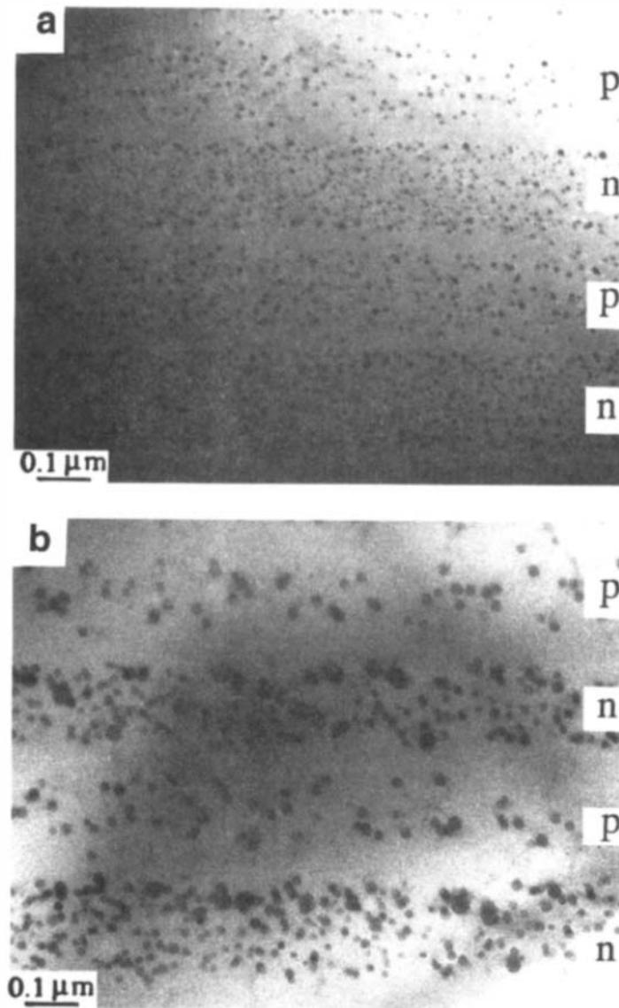
Figure 5 TEM image of a series of 200-nm GaAs regions uniformly doped with Si at  $1 \times 10^{18}$  cm $^{-3}$  followed by a 200-nm GaAs region uniformly doped with Be at  $1 \times 10^{18}$  cm $^{-3}$ , and subsequently annealed at (a) 700°C for 30 s and (b) 900°C for 30 s.
