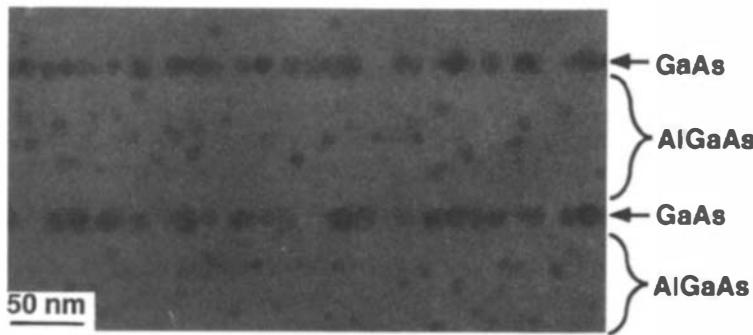
*Figure 8* Bright-field image of 10-nm thick GaAs wells separated by 100-nm AlGaAs barriers for samples annealed at 700°C for 5 min.
