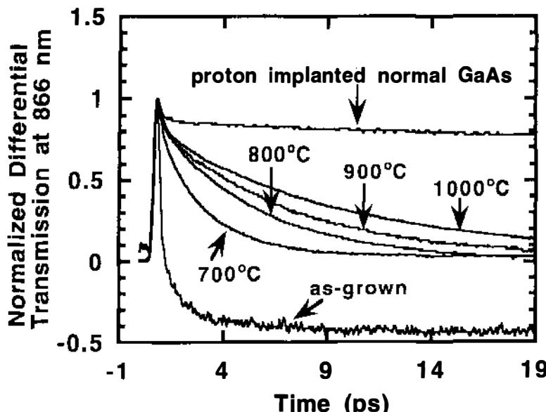
**Figure 30** Normalized differential transmission measurements of low-temperature-grown GaAs showing the dependence of the decay of the differential transmission on the arsenic cluster coarsening anneal. The anneals were of duration 30 s at the temperatures indicated. The normal GaAs film is 1- $\mu\text{m}$  MBE material implanted with  $1 \times 10^{12} \text{ cm}^{-2}$  protons in order to assure recovery to equilibrium between laser pulses.
