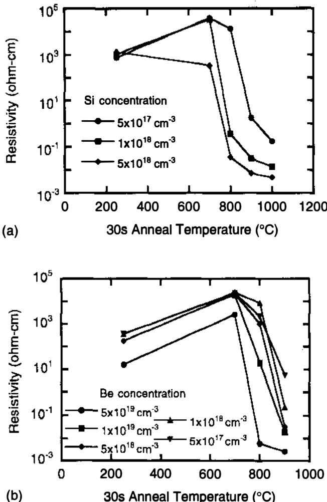
Figure 11 Resistivity as a function of temperature for 30-s isochronal annealing of GaAs epilayers containing excess arsenic for (a) three different *n*-type doping concentrations, and (b) five different *p*-type doping concentrations.
