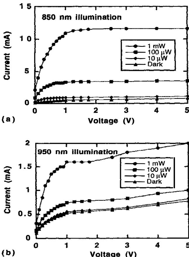
Figure 34 Current-voltage characteristics of the Figure 23 photodetector with 1-μm finger spacing under (a) 850- and (b) 950-nm illumination.
