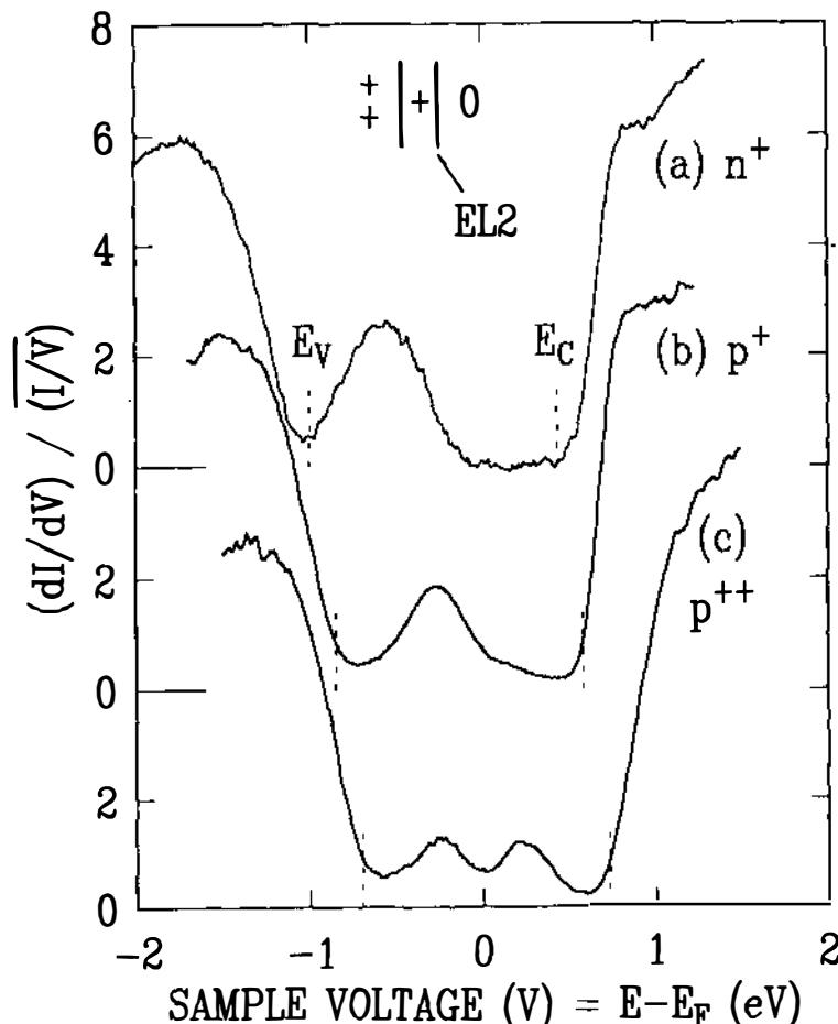
Figure 23 Tunneling spectra acquired from layers of as-grown LTG-GaAs containing varying amount of compensating shallow dopants. The valence-band maximum  $E_V$  and conduction-band minimum  $E_C$  are indicated by dashed lines in each spectrum. An intense band of states, arising from arsenic-related defects, appears within the band gap. The states of a bulk arsenic antisite defect (EL2) are shown in the upper part of the figure, relative to the band edges of spectrum (a).
