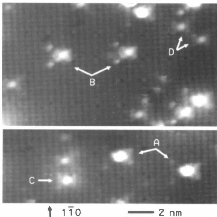
Figure 22 STM images of the (110) cleaved surface of as-grown LTG-GaAs, acquired with 0.1 nA tunnel current and at a sample voltage of –2.0 V. Various point defects can be seen, classified as types A, B, C, and D, as indicated.
