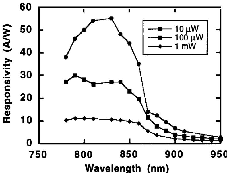
Figure 35 Responsivity vs wavelength of the Figure 23 photodetector with optical power as a parameter.
