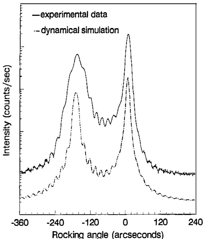
Figure 1 Experimental and calculated (004) double-crystal rocking curves for LTG-GaAs sample containing 1.5% excess arsenic.
