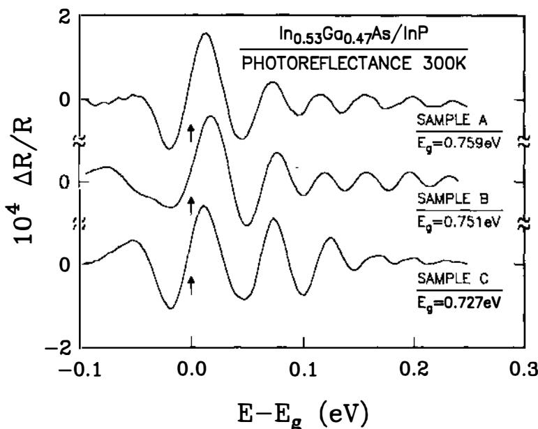
Figure 21 Photoreflectance spectra at 300 K for two ALTUN (samples A and B) and one UP (sample C) GaInAs/InP materials plotted as a function of  $(E-E_g)$ .
