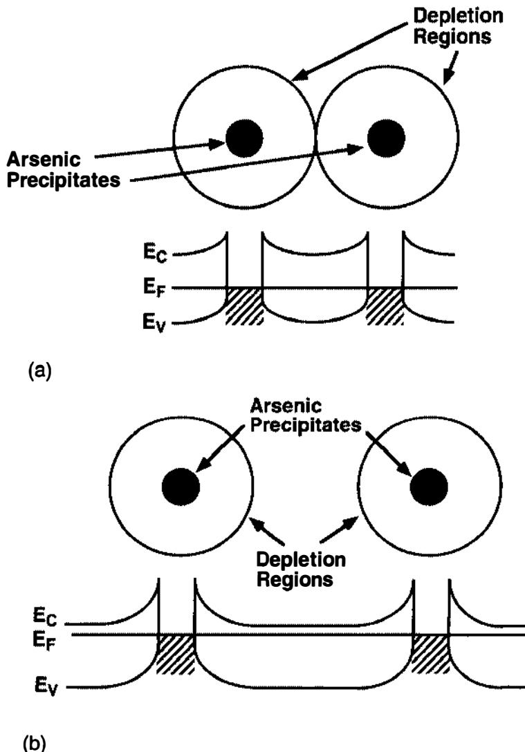
Figure 10 (a) Depletion regions around arsenic precipitates such that the depletion regions just overlap. (b) Depletion regions around arsenic precipitates with spacing such that there is undepleted material between the precipitates.
