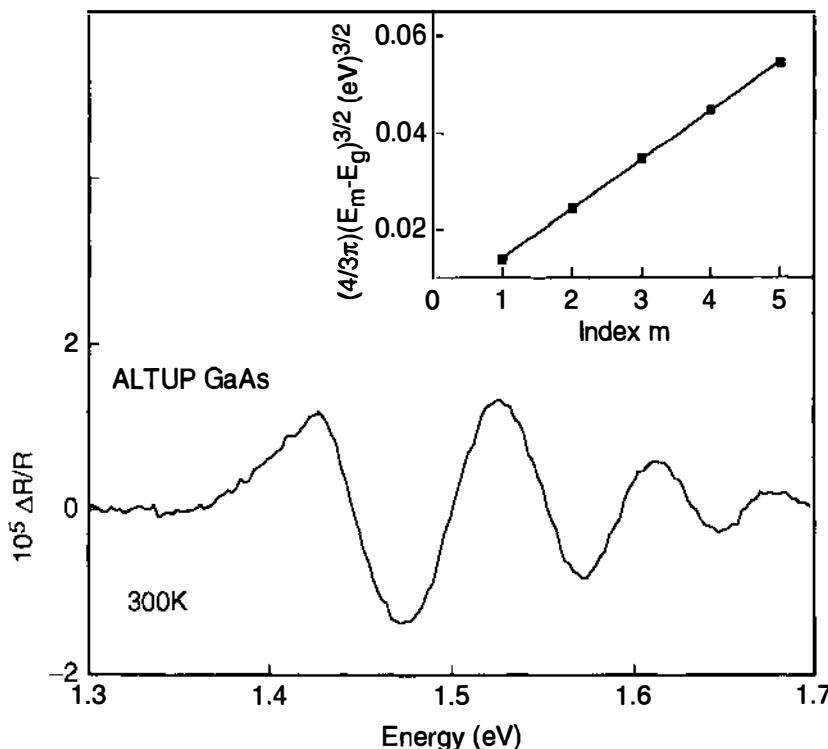
Figure 19 Contactless electroreflectance spectrum from the ALTUP structure at 300 K. The inset shows a plot of  $(4/3\pi)(E_m - E_g)^{3/2}$  as a function of the Franz-Keldysh oscillations extrema index  $m$ .
