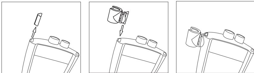
The FiveGo™ clip (Part no.51302960) is an electrode holder that can be placed next to the display on either side of the housing. To mount the clip, remove the cover from the clip's fixing point. Attach the clip by pressing it into the recess. Slide the shaft of the sensor into the clip from above.
