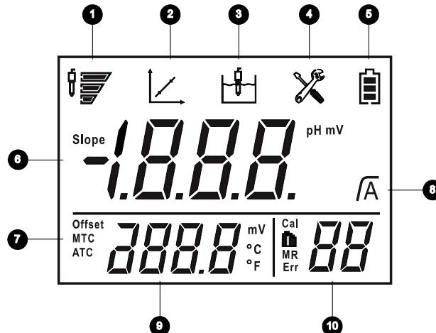
**1** Electrode condition (For electrode maintenance see section 5.2)
