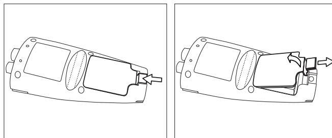
1. Pull the fixing point of the battery cover in the direction of the arrow, hold the lid with two fingers and remove it;
