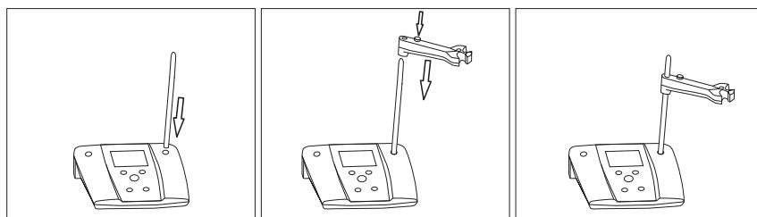
1. Remove the electrode stand rubber cover on that side of the bench meter where you prefer the stand.
