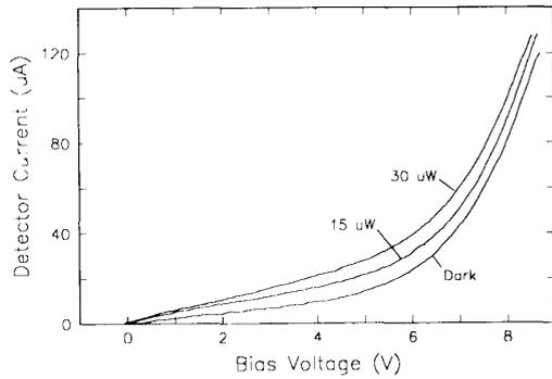
Fig. 2. Responsivities of the IMSM detector at 0, 15, and 30  $\mu\text{W}$ .
