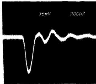
Fig. 3. Optical pulse response of the detector. FWHM = 140 ps and bandwidth = 3.2 GHz.
