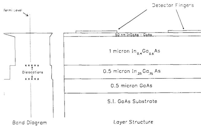
Fig. 1. The layer structure of the photodetector.
