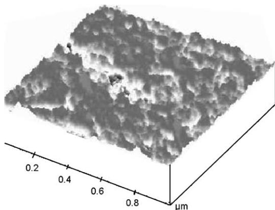
Fig. 4. AFM image of InP/GaP wafer with surface roughness of 2.48 nm.
