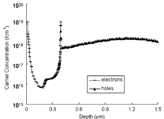
Fig. 5. ECV carrier concentration profile of InP/GaP photodiodes as a function of device depth.
