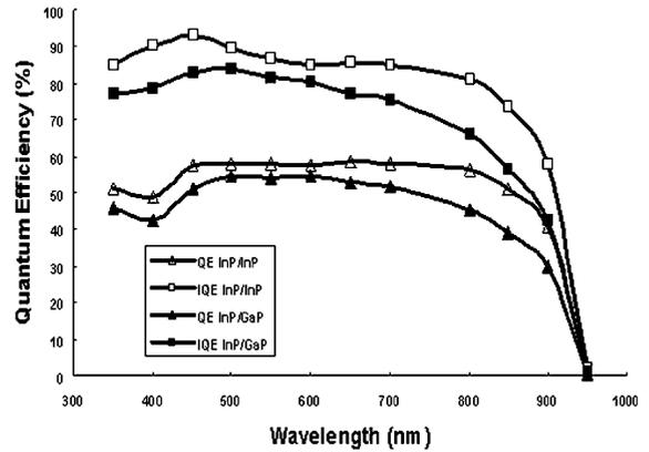
Fig. 7. Quantum efficiency as a function of photon wavelength for drift dominated InP/GaP photodiodes and InP/InP devices.
