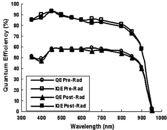
Fig. 1. Quantum efficiency versus photon wavelength for drift dominated InP solar cells before and after irradiation with  $10^{15} \text{ cm}^{-2}$  1 MeV electrons.
