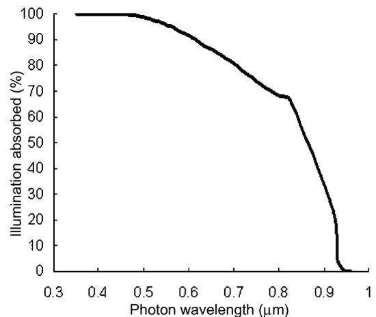
Fig. 3. The percentage of illumination absorbed in InP of 350 nm as a function of photon wavelength.
