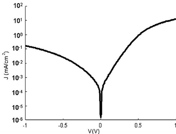
Fig. 6. Dark current density–voltage characteristics of drift dominated InP/GaP photodiodes.
