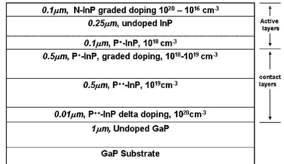
Fig. 2. Schematic layer structure of drift dominated InP/GaP photodiodes.
