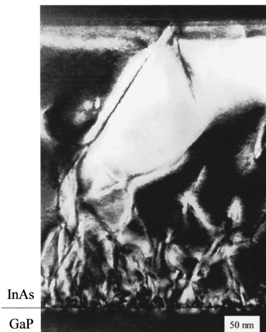
FIG. 1. A cross sectional TEM image of a 0.5 \mu\text{m} InAs film.
