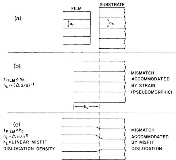
FIG. 1. A schematic representation of the formation of misfit interfaces.
