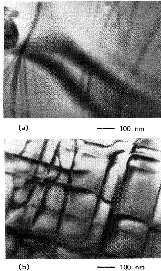
FIG. 2. Transmission-electron photomicrographs of the pseudomorphic interface of sample 1 [Fig. 2(a)], and the interface of sample 2 containing misfit dislocations [Fig. 2(b)].
