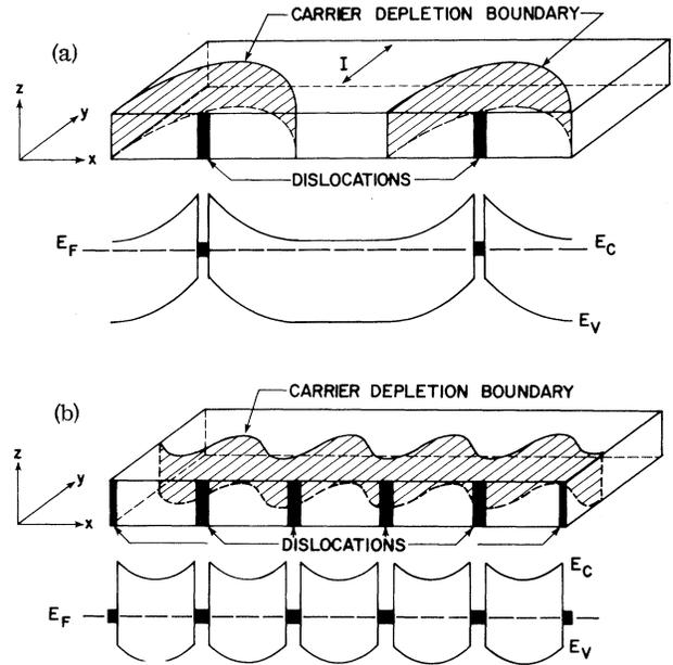
FIG. 4. A schematic representation of the expected electronic behavior of misfit dislocations. (See text for detailed description.)
