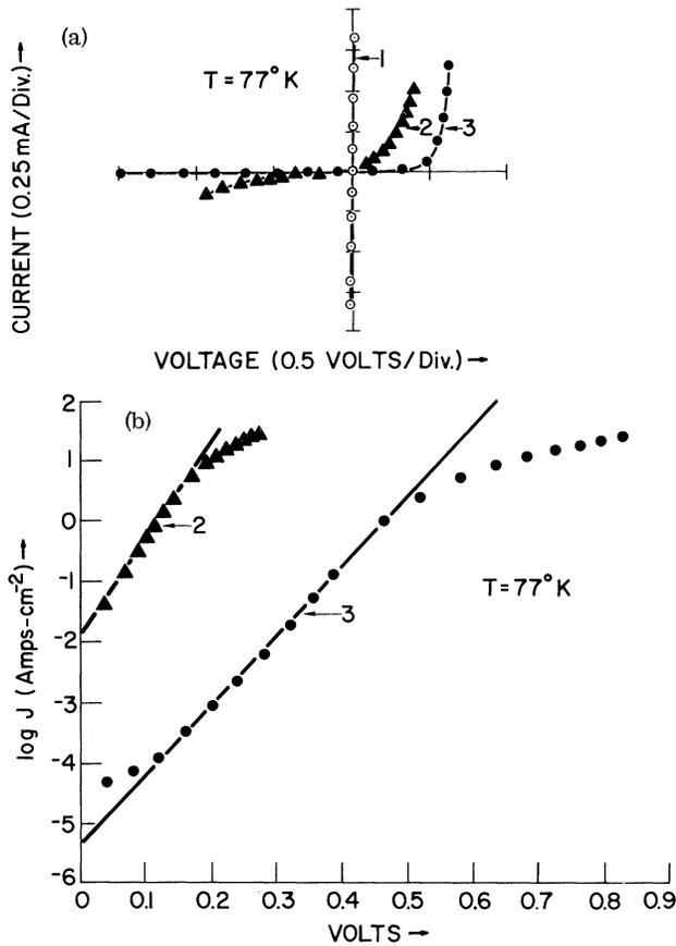
FIG. 3. Current-voltage measurements of three different GaInAs/GaAs interfaces (1, 2, and 3), with cross section  $1.2 \times 10^{-4} \text{ cm}^2$ . (See text for detailed description.) In (b), the GaInAs is biased positive with respect to the GaAs.
